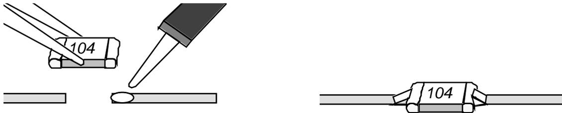
Use a 1.6mm tip (or smaller) and 26 gauge solder (0.5mm). Thicker solder or tips give enormous problems. Do the soldering as quickly as possible to avoid separating the end contact from the component. Don't worry about what the solder joint looks like. The strength of joint is unimportant.
