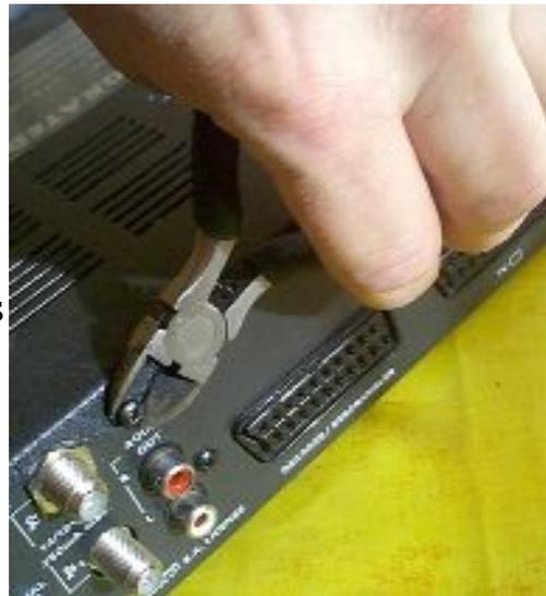
but some manufacturers use two-piece plastic rivets. The trick is to lift the “mushroom” head of the rivet up with cutters. You can then grip the lower body of the rivet and lift it out.
