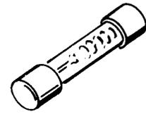
A fuse marked "T1A" is a one amp fuse with a Time-delay action. A fuse marked "F1A" is a one amp fuse with a Fast action.
