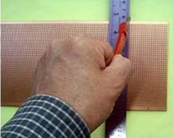
Once the circuit is proven you can build it up. This project is easy to build on perforated stripboard. We'll call it by a well known manufacturer's trademark "Veroboard®".
