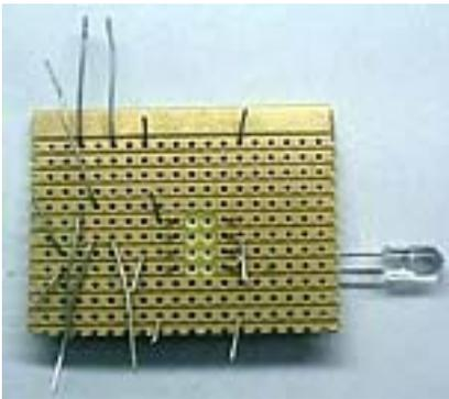
Bend the component wires underneath the board as you fit each part. This will prevent them from falling out as you fit subsequent parts to the board. At this stage it is easy to pull out parts and reposition them if you don't like the initial result.
