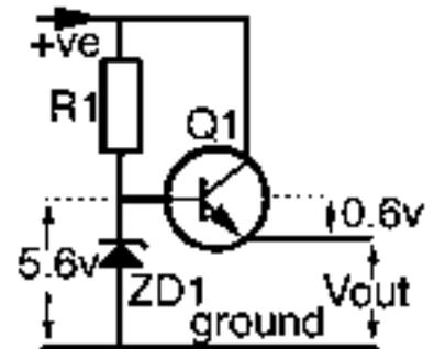
It is easy to calculate. The voltage at Q1 base connection is 5.6 volts.
