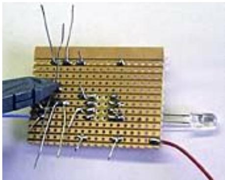
When you are happy that you have positioned the components and link wires correctly, solder the wires to the copper tracks. First, be sure to apply fresh solder to the
