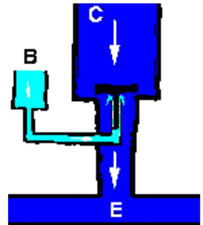
2. The amount of current that can flow from "C" to "E" is limited by the "pipe diameter". So, no matter how much current we push into "B", there will be a point beyond which we can't get any more current flow from "C" to "E". The only way to solve this problem is to use a larger transistor. A "power transistor". This tends to have a lower "gain" so is less efficient.
