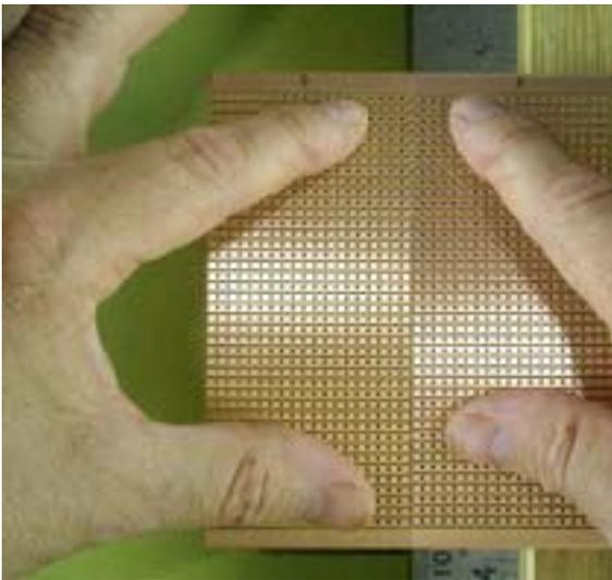
Now rest the board over the edge of a table or bench, with a steel ruler or similar sharp edge immediately below the score mark. Apply downward pressure and the end piece should snap off cleanly.
