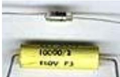
Polystyrene film capacitors used where a small capacitance is needed with low tolerance spread (2% or better) and good temperature stability. Drawbacks include relatively high inductance and cost and susceptibility to cleaning solvents. Yellow example is of the "extended" type which is better sealed against ingress of liquids. Polystyrene capacitors are most often used in tuned circuits (oscillators and filters) where frequency stability is important.
