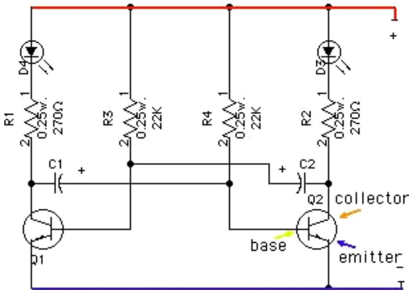
Back to basics. You can build lots of interesting and useful circuits without using I.C.s. After all, an I.C. is simply a handy container for a bunch of miniature components! Here is an extremely common circuit with a multitude of uses - eg. a slow alternating flash for a model railway crossing or a fast rate of flash for a flickering flame.
