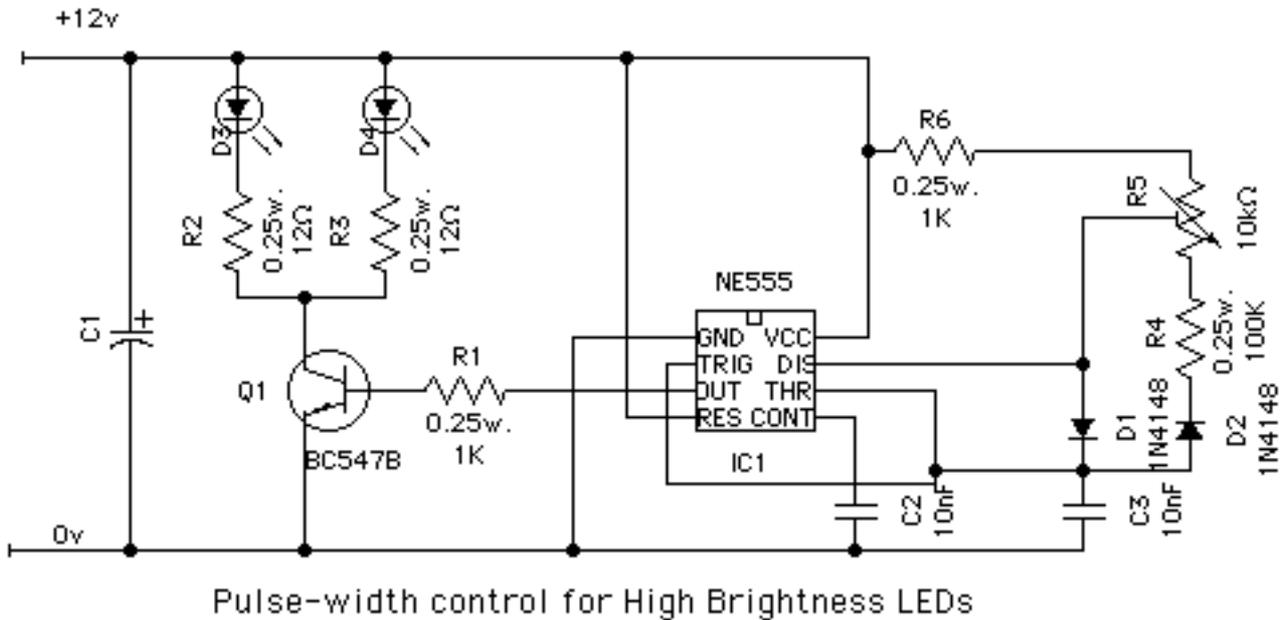
Pulse-width control for High Brightness LEDs
