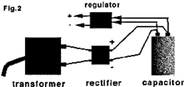
There are several ways but the simplest is to use a transformer to reduce the voltage to, say 12 volts a.c. (Fig.2) This lower voltage can be fed through a "rectifier" which
