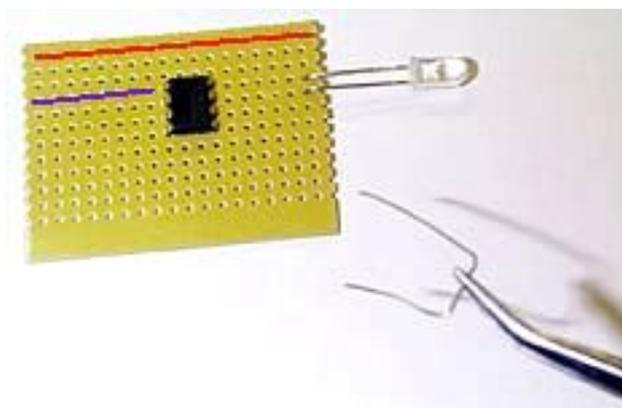
Look at the circuit diagram and decide where the parts can fit. The LED connects between pins 7 and 8 so that's easy to do. Wire links are used to connect pins to other tracks. At this stage you should choose where the **positive** and **zero voltage** tracks can be. I've marked my choice with red and blue lines, respectively. Needle-nose pliers or tweezers are handy for bending and fitting the wires.
