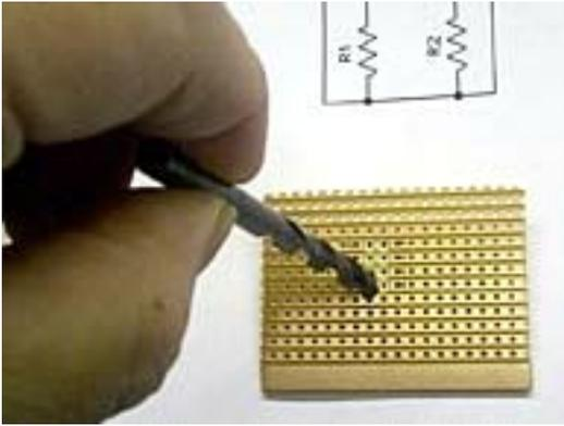
Once you are happy that the I.C. is in a convenient position, you can cut the copper tracks between its two rows of pins, otherwise they will be connected together. This operation is carried out simply by using a twist drill of 3.5 - 4.0 millimetres in diameter. Make sure each track is cut completely. If you are unsure of the I.C. position, leave this operation till later, but do it before you solder the I.C. pins.
