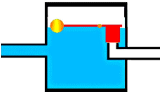
However, if there is a steady current, only the initial short burst will flow until the "floating ball valve" closes and stops further flow.
