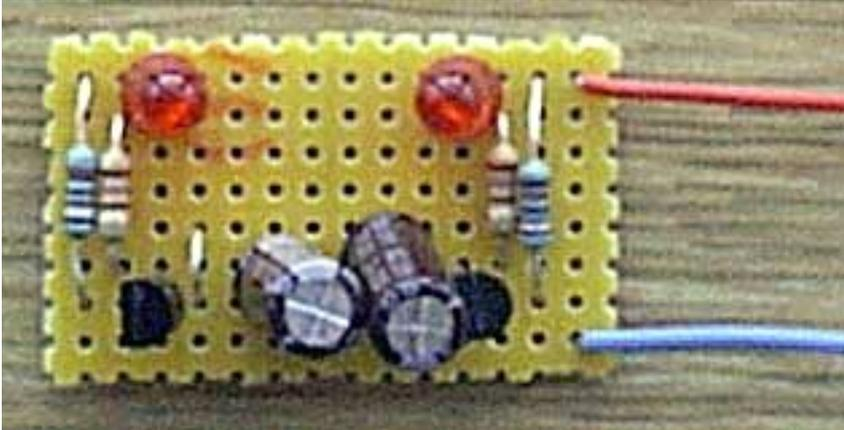
Here are the components soldered onto Veroboard, The layout follows the circuit diagram fairly closely but the crossed-over capacitors are dealt with by adding a wire link. Three tracks have to be cut (highlighted in yellow).
