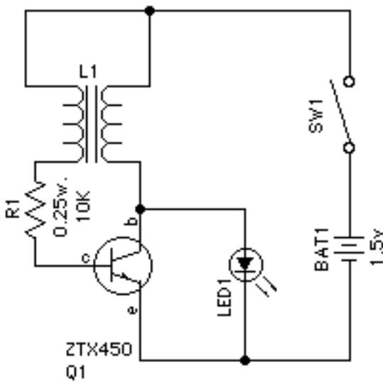
Running an LED off just 1.5 volts to make a Micro-torch
