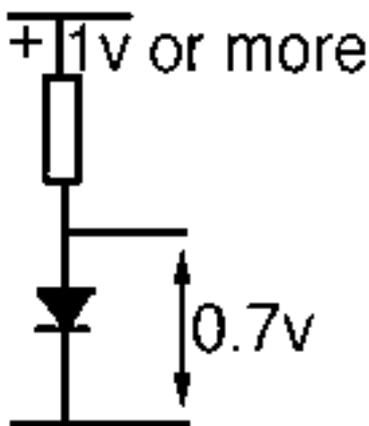
**Silicon** diode = 0.4 to 0.7v dependent on type
