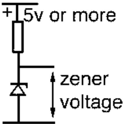
Zener diodes are used to "clamp" a voltage in order to prevent it rising higher than a certain value. This might be to protect a circuit from damage or it might be to "chop off" part of an alternating waveform for various reasons. Zener diodes are also used to provide a fixed "reference voltage" from a supply voltage that varies. They are widely used in regulated power supply circuits.
