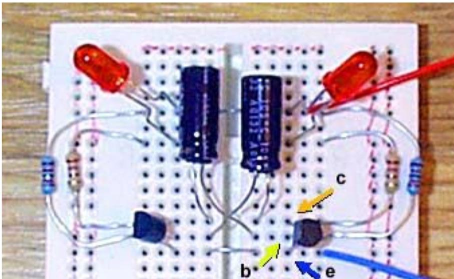
the “collector”, the “base” and the “emitter”. I’ve marked these with arrows. (Please note that all BC transistors are configured like this but 2N devices may have the collector and base transposed). Resistors R1 and R4 protect the LEDs from excessive current. The actual value is dependent on the characteristics of the
