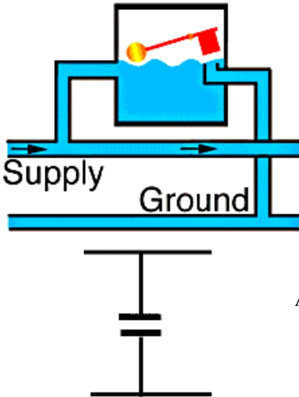
Where a capacitor is used to decouple a circuit, the effect is to "smooth out ripples". Any ripples, waves or pulses of current are passed to ground while d.c. flows smoothly.
