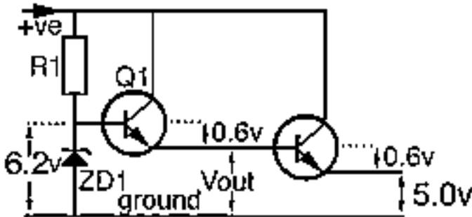
The first circuit can be improved upon to provide more current. All we need to do is to add a second transistor (which has a higher rating to handle the extra current) and change the zener diode to clamp at 6.2 volts in order to compensate for the b-e voltage of BOTH transistors.
