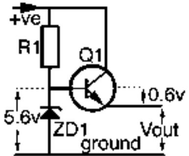
For the zener diode let's choose a BZX55C5V6. This will need a minimum of 10mA of current to produce a stable voltage. So Q1 requires 1mA, ZD1 requires 10mA, making a total of 11mA through R1.
