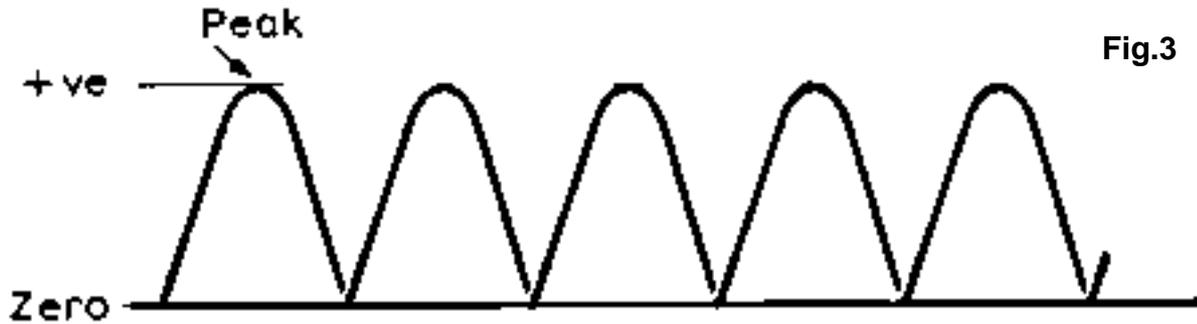
The first step is to connect a large value capacitor to the output of the rectifier. A capacitor acts as a voltage reservoir and has the effect of smoothing the "ripples". This is still not the same as a battery produces but it's often good enough for charging batteries
