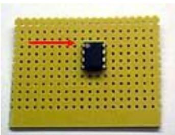
Fit the I.C. in a roughly central position and bend its pins to retain it. Pin 1 is indicated by **the arrow**. Pin 1 normally has a dot or notch just to the right of it. The other pins are numbered clockwise from 1.
