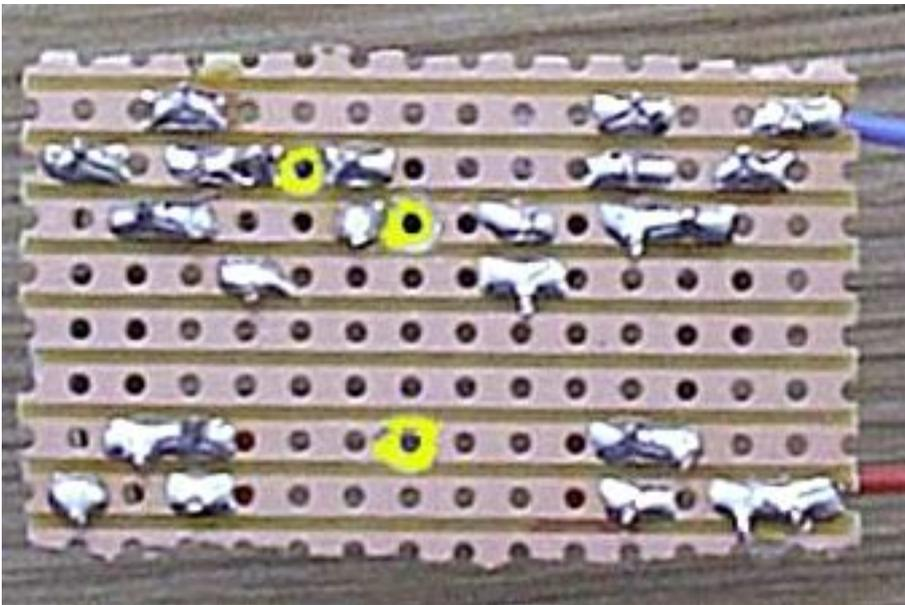
I have pushed the LEDs down onto the board but you might prefer to leave them “on stalks”. This leaves them prone to vibration-fracture so it’s a good idea to squirt some hot-melt adhesive around the wires to secure them to the board. If you leave the LED wires long, it’s easier to fit the unit into, say, a robot with “flashing eyes”.
