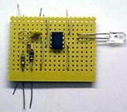
Carry on fitting the components. The actual physical positions of the parts are unimportant. Just make sure that they will be connected to each other and to the I.C. pins in accordance with the circuit diagram. The physical layout of parts on the board doesn't have to look exactly like the circuit diagram, although it may help you if it is reasonably close. For a more complex project, you may find it easier to sketch a provisional component layout on squared paper.
