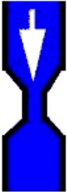
Imagine water flowing through a pipe. If we make the pipe narrow then this will restrict the flow of water. If we force the water (current) through the narrow gap by increasing the pressure (voltage) then energy will be given off as heat. In addition, there will be a significant difference in pressure (voltage) above and below the restriction. As an example, imagine pumping up a tyre by hand. The narrow pipe of the pump gets hot doesn't it?
