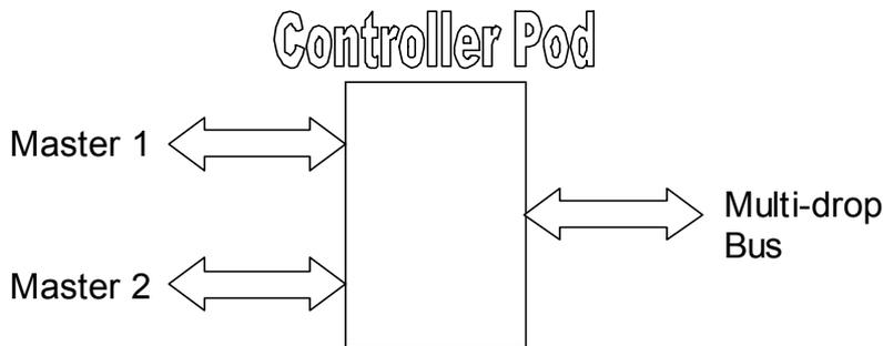
Due to the complexity of multi-master systems, it can be preferable to use a multi-master controller pod sitting on the cctalk bus to arbitrate between 2 or more master devices. The controller pod can assign priorities to the various serial commands and deny one master access to the bus when another is waiting for a reply. For this purpose, a *BUSY* return message has been defined. If a master receives a *BUSY* response, it must retry after a ( preferably random ) amount of time.
