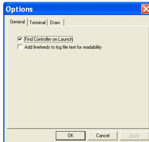
**Find Controller on Launch** -- If checked, the SDU looks for a USB driver, a Serial driver, and then a touch controller on any available COM port. The SDU tries to identify the controller. If a controller is found, details are displayed about the driver or the COM port, and the controller.
