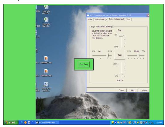
Determine if the area you have defined is sufficient for your needs. Can you touch into the corners and along the edges of the sensor? Click Escape, End Test, or Return to go back to the Edge Adjustment tab. If you are satisfied with the selections you have made – you are done. If not, adjust the sliders to better accommodate your needs.
