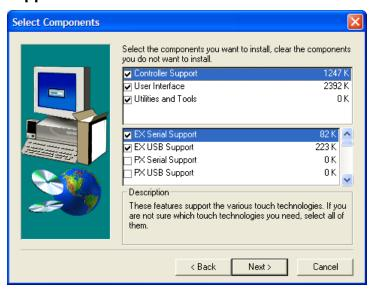
Various controller support is available. By default, all controller support is installed. If you do not want to support a specific controller, deselect that component in either the upgrade or custom setup screens.
