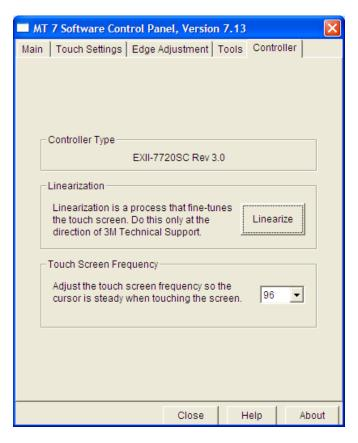
The Controller tab contains different choices depending on the type of touch controller(s) you have attached to your system and which options you selected from the Advanced Options from the Tools tab.
