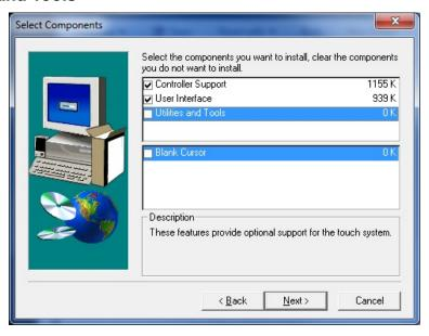
This option enables you to hide the cursor. By selecting this, MT 7 Software installs a blank cursor on your system. To always hide the cursor, open the Windows<sup>TM</sup> Control Panel, select mouse settings and then browse to the MicroTouch folder and select blank cursor.
