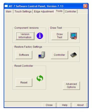
The Tools tab enables you to perform a variety of diagnostics to optimize the performance of your touch sensor. This tab is also the gateway to advanced touch options.
