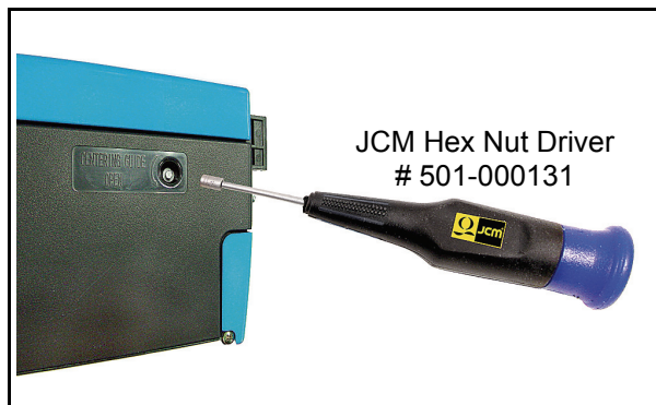
Figure 2-14 Opening UBA Centering Mechanism
