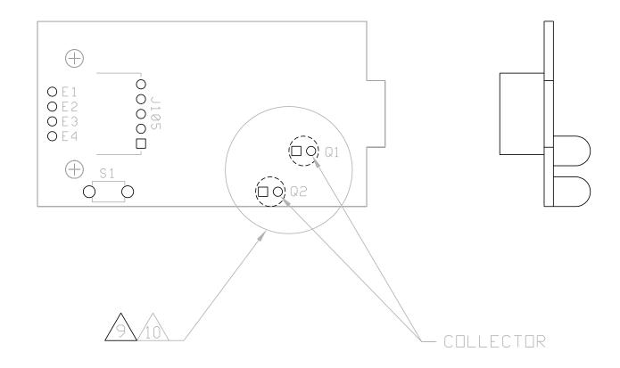
DO NOT ALLOW OPTICAL DEVICES TO COME IN CONTACT WITH ANY CHEMICALS WHICH COULD ALTER THEIR OPTICAL CHARACTERISTICS.
