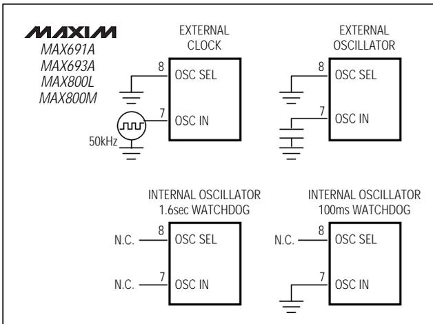
Figure 3. Oscillator Circuits
