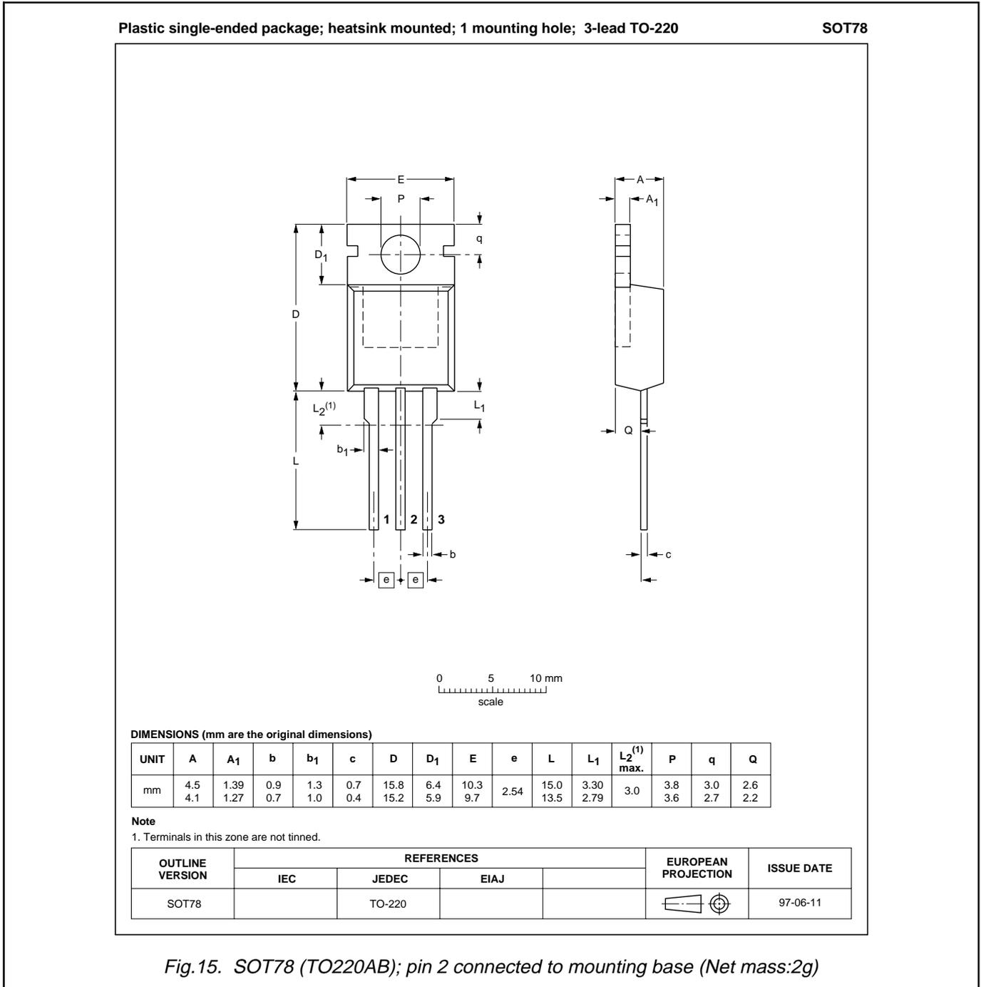
Fig. 15. SOT78 (TO220AB); pin 2 connected to mounting base (Net mass:2g)
