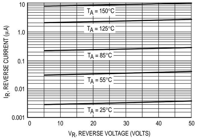
**Figure 3. Leakage Current**
