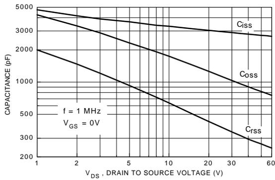
**Figure 9. Capacitance Characteristics**
