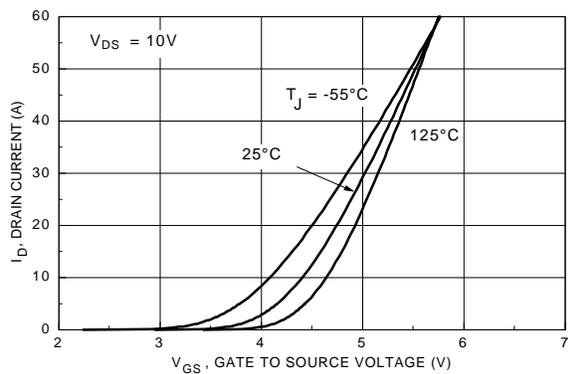
Figure 5. Transfer Characteristics
