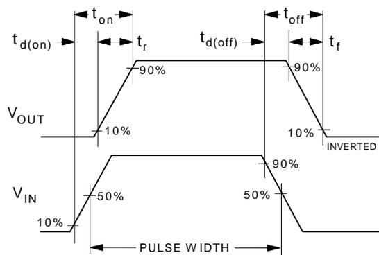
**Figure 12. Switching Waveforms**
