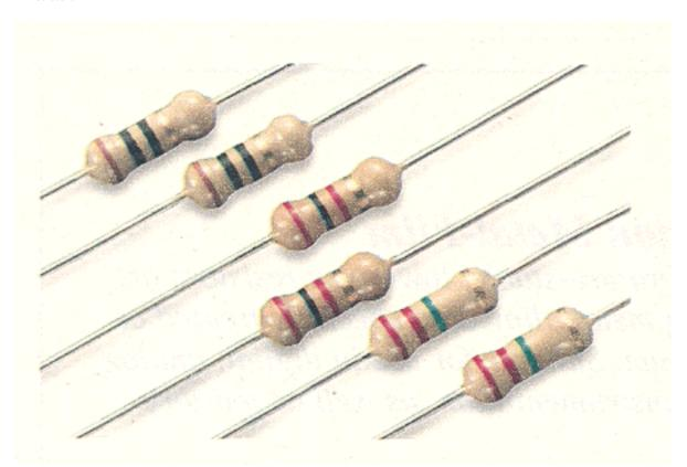
Similar in appearance is the 1% resistors. Four colored stripes are used to indicate the resistance value instead of using three colors 2& or 5% values use. The last band is Brown, indicating a 1% resistor.
