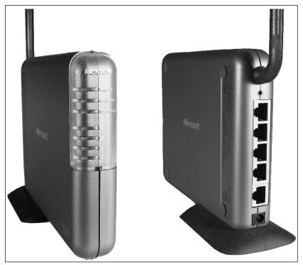
**Figure 12-5:** Microsoft model MN-700 IEEE 802.11g base station ©2004 Barry Press & Marcia Press
