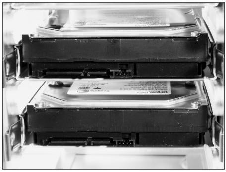
**Figure 25-4:** Disk drives mounted in chassis ©2004 Barry Press & Marcia Press
