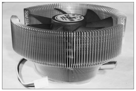
**Figure 25-10:** Zalman processor cooler ©2004 Barry Press & Marcia Press
