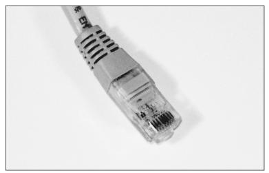
**Figure 12-1:** RJ-45 connector on Ethernet cable ©2004 Barry Press & Marcia Press
