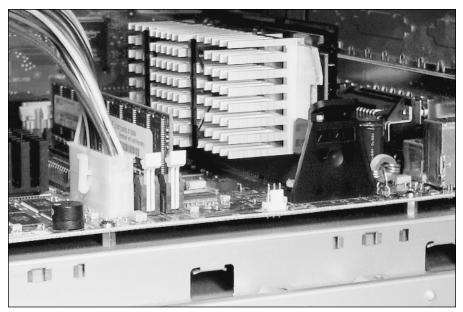
Figure 25-14: Main ATX power supply cable ©2004 Barry Press & Marcia Press
