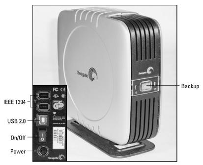
**Figure 10-4:** USB-connected external hard disk drive ©2004 Barry Press & Marcia Press
