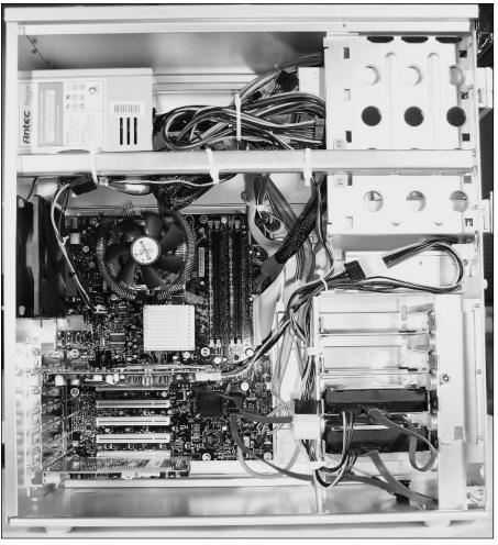
**Figure 25-21:** Completed system internal view ©2004 Barry Press & Marcia Press
