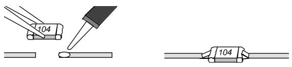
Use a 1.6mm tip (or smaller) and 26 gauge solder (0.5mm). Thicker solder or tips give enormous problems. Do the soldering as quickly as possible to avoid separating the end contact from the component. Don't worry about what the solder joint looks like. The strength of joint is unimportant.
