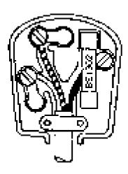
The green-yellow earth wire (if present) is deliberately left long so that, if someone should trip on the cable or tug at it in such a way as to pull the sheath out of the clamp, the safety earth will always be the *last* wire to be disconnected, thus ensuring that the appliance is earthed while there is a possibility of its becoming "live".
