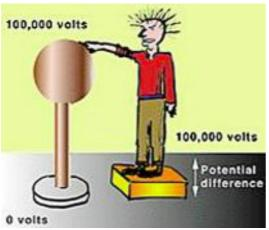
You have probably all seen a Van de Graaf generator at school or at science fairs. It has a moving rubber belt which transfers electrons from its base to a metal globe. If you touch the globe you will receive an electric shock because your feet are on the ground at zero voltage and your hand is touching the globe (not for long!) at 100,000 volts. The potential difference between your feet and hand is 100,000 volts.
