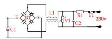
The sketch shows a typical power supply mains input section. 230 volt AC mains comes in via R1 (a resistor to limit voltage surges. C2 removes both incoming and outgoing interference, as does the double filter L1. V1 is a "varistor" which is sometimes fitted. It looks like a "smartie" or "M&M" and normally has no effect. However, if a high voltage surge comes from the mains supply, the varistor conducts heavily, causing the fuse F1 to melt and, hopefully, protecting the equipment from excessive
