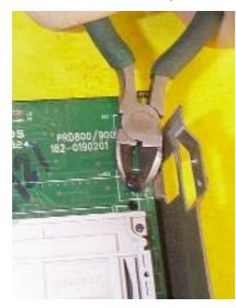
Once the cover is off you have the problem of removing the board assembly. Screws are usually obvious
