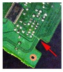
cornered cut-out in the printed circuit board can develop a crack, which may propogate through several copper tracks. If you suspect that a crack is present, put your meter on the diode test range or "bleep" range and put the probes on solder pads, one on each side of the suspected crack - or use a sharp blade to scrape away the green resin to expose bare copper. Some cracks will give a good continuity reading until the board is flexed or warmed up with a hair dryer. Some cracks show up only
