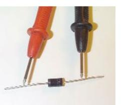
between 0.2 and 0.7 volts, dependent on the type of diode. More importantly, with the probes reversed, the reading should indicate infinity because no current should flow in the reverse direction. If the diode gives a low reading in both directions then it is no longer a diode!
