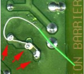
both sides. If possible, kink the component lead above the board to minimise movement. If there is no solder pad near the break, use a sharp blade to scrape the green solder-resist varnish off the copper track. apply a little solder, quickly, to tin the bare copper track. Now solder the wire along the track so the crack is bridged and cut off any excess wire.
