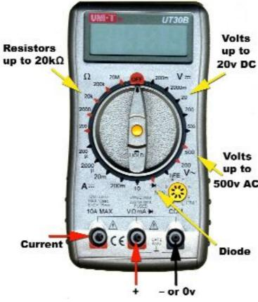
A multimeter has a selection of "ranges". The most commonly used ranges are indicated here by yellow arrows. Most **DC voltages** in electronic equipment are below 40 volts (for safety). This particular meter has a choice of ranges for measuring up to 200 500v AC milliVolts (thousandths of a volt), up to 2 volts, up to 20 volts, up to 200 and up to 500 volts. Of these, the 20 volt DC range is the most useful one. If the actual voltage is between 2 volts and 20 volts then
