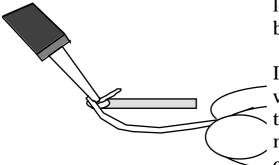
lead and push it upright so that it can be removed easily from the hole.
