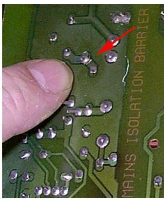
the wire inside has melted. If it looks all right, don't believe your eyes. Measure it. It should read almost short-circuit - after all, it's only a piece of thin wire inside a tube.
