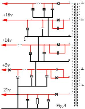
the diodes from **fast-risetime pulses**. Some electrolytics also have low value **ceramic capacitors** connected across them to remove fast-risetime pulses.
