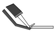
internal spring. You prime the sucker by pushing the plunger down until it locks. Pressing a button releases the springloaded plunger and it sucks up anything close to its nozzle. Great for zits! Not so great for printed circuits. The usual effect
