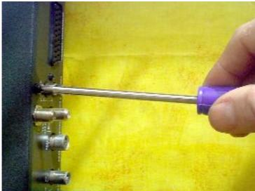
Most receivers are held together with cross-head screws. dependent on where they were assembled, these screws could be either "Philips" or "Posidrive". It's most important that you select the correct screwdriver, otherwise you may damage the slots and make the screw difficult to remove.
