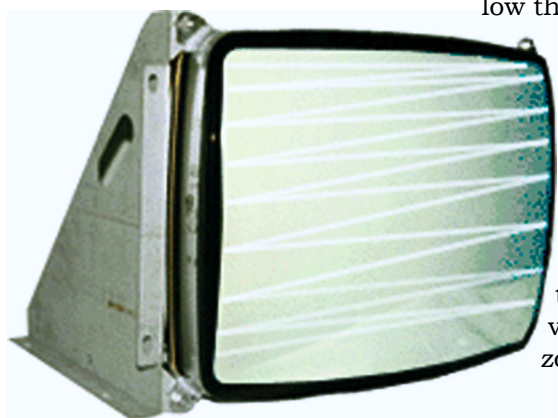
Blanking failure causes white, vertical retrace lines to appear on the screen.
