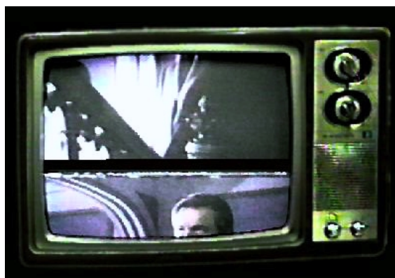
Vertical sync prevents the picture from rolling as shown here.
