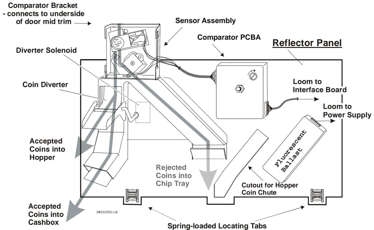
Figure 6-1 CC-62 Coin Chute Assembly - Location
