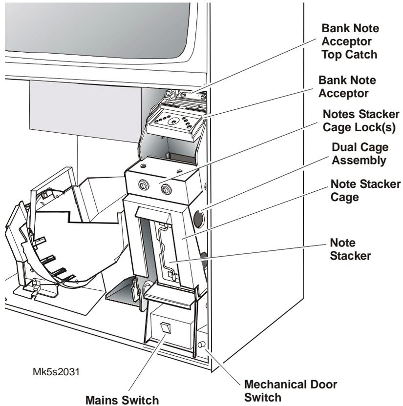
Figure 9-1 Bank Note Acceptor Location
