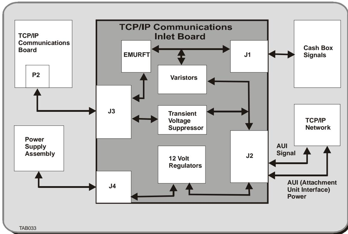
Figure 16-5 TCP/IP Comms Inlet Board - Block Diagram
