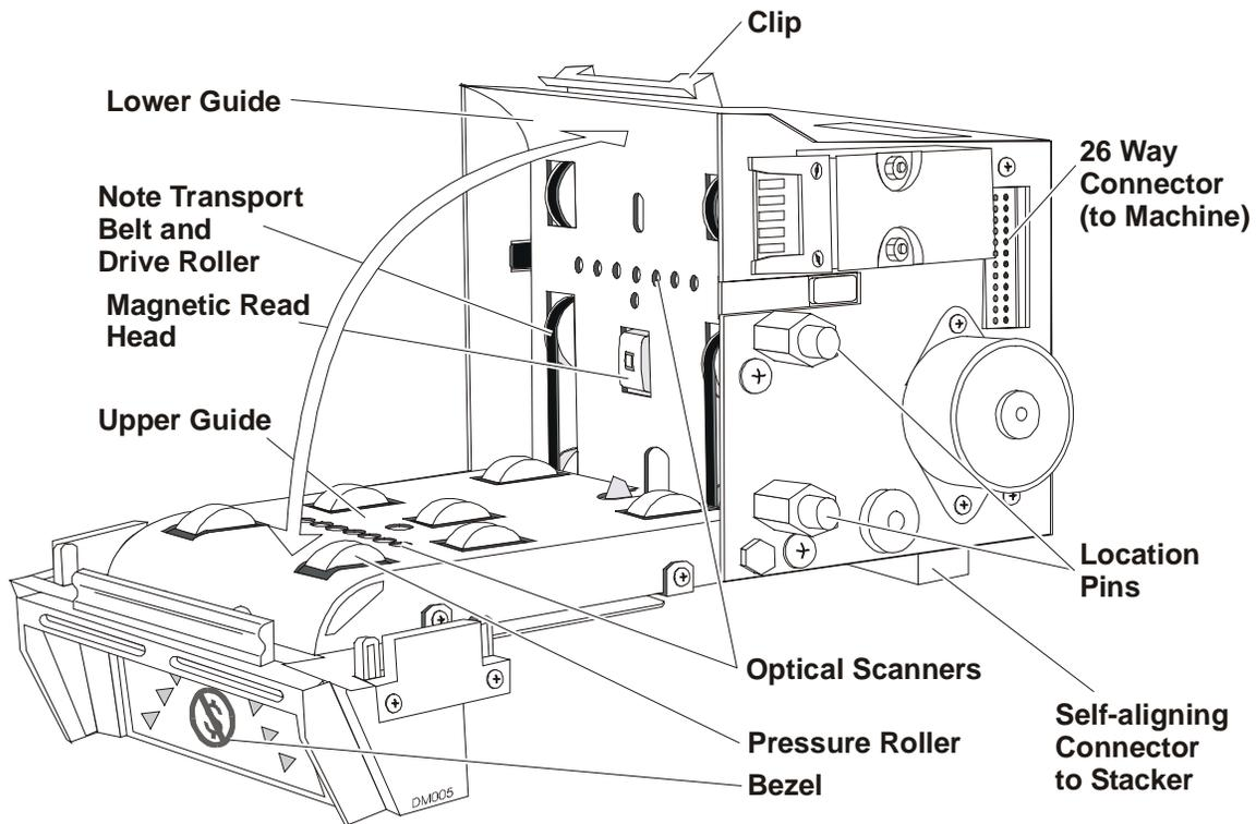
Figure 9-2 Bank Note Acceptor with open Upper Guide
