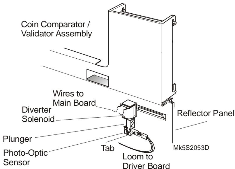
Figure 6-14 Diverter Solenoid and Photo-Optic Sensor
