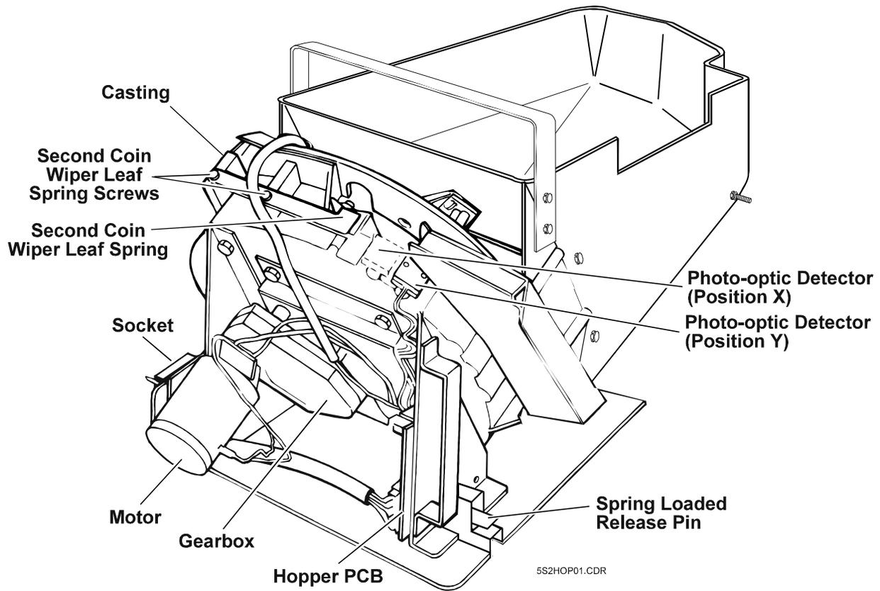
Figure 7-2 Hopper- rear view
