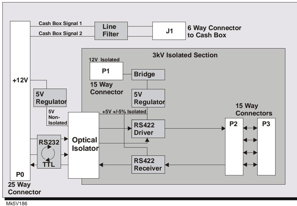
Figure 16-1 VLC Comms Inlet PCB Block Diagram
