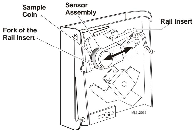
Figure 6-4 CC-62 Sensor Assembly
