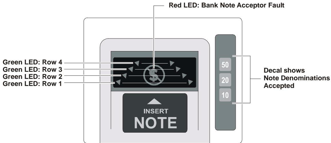
Figure 9-10 Bezel Assembly Indicators - LED Displays
