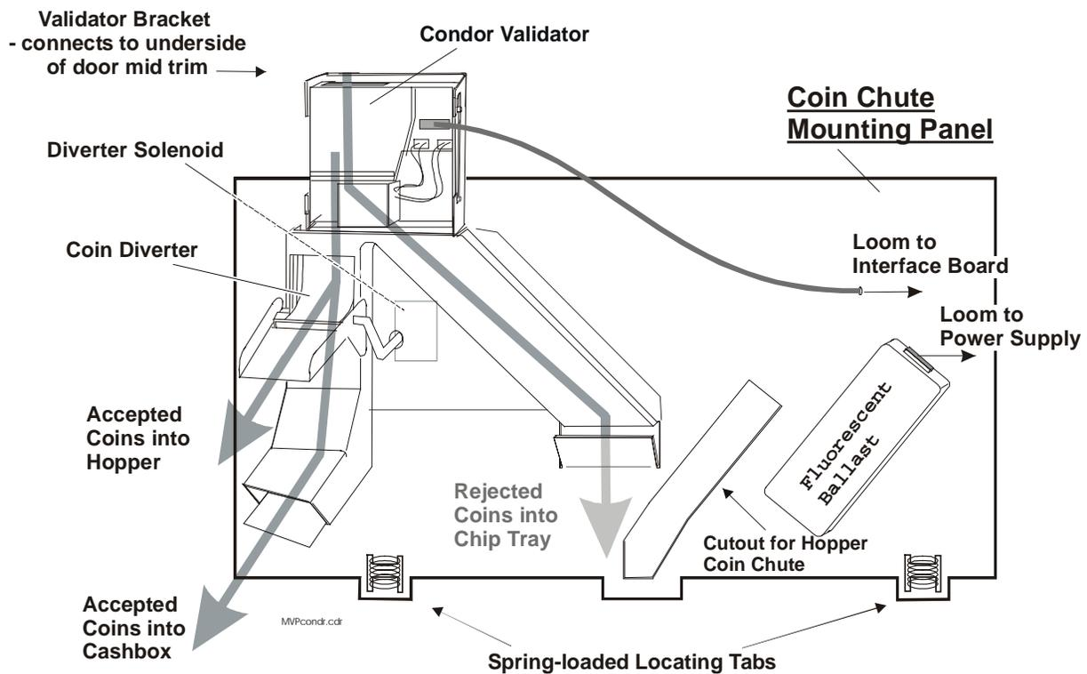
Figure 6-7 Condor Coin Handling Assembly
