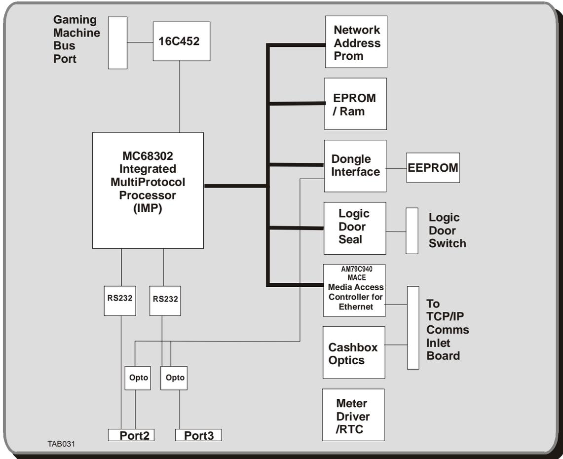
Figure 16-3 TCP/IP Communications Board - Block Diagram
