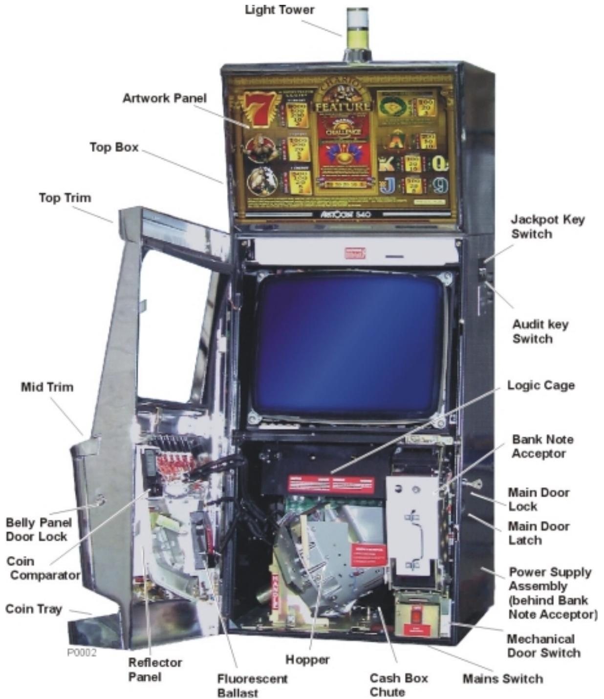
Figure 1-2 Typical MVP Video Gaming Machine with Bill Acceptor
