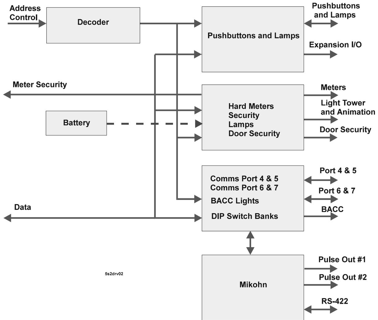
Figure 13-4 Extended US I/O Driver Board Block Diagram
