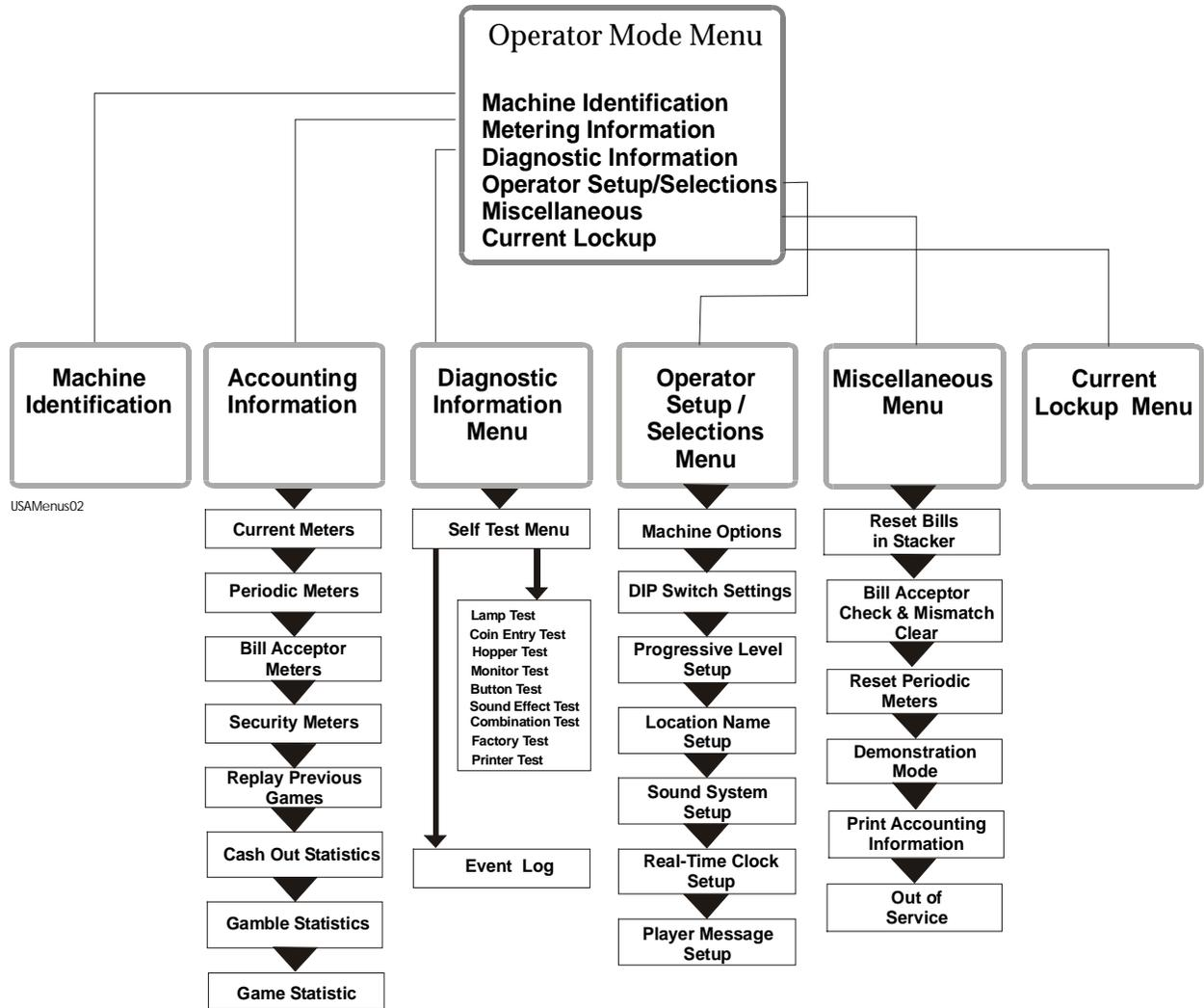
Figure 3-4 Operator Mode Menu Displays - Typical Structure
