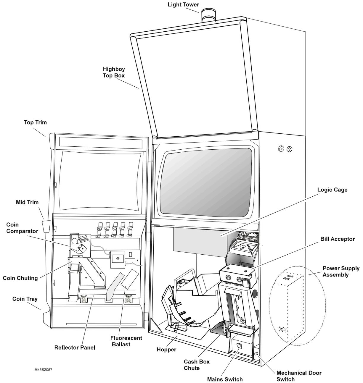
Figure 4-2 MVP Gaming Machine with Highboy Top Box and Bill Acceptor
