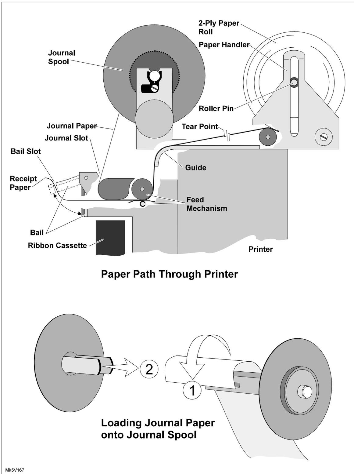
Figure 8-4 Replacing the Paper Roll
