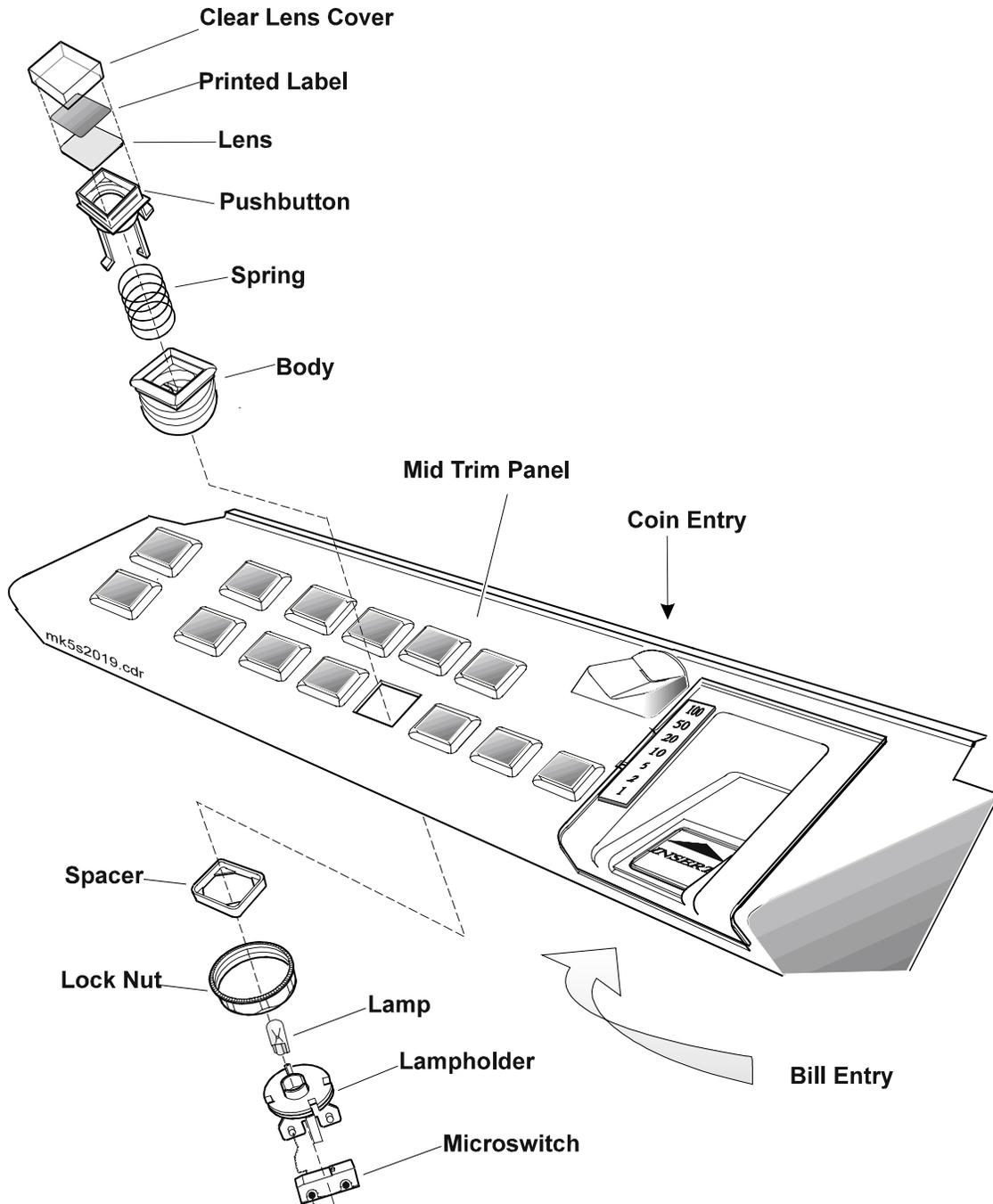
Figure 4-7 Playbutton: Exploded View
