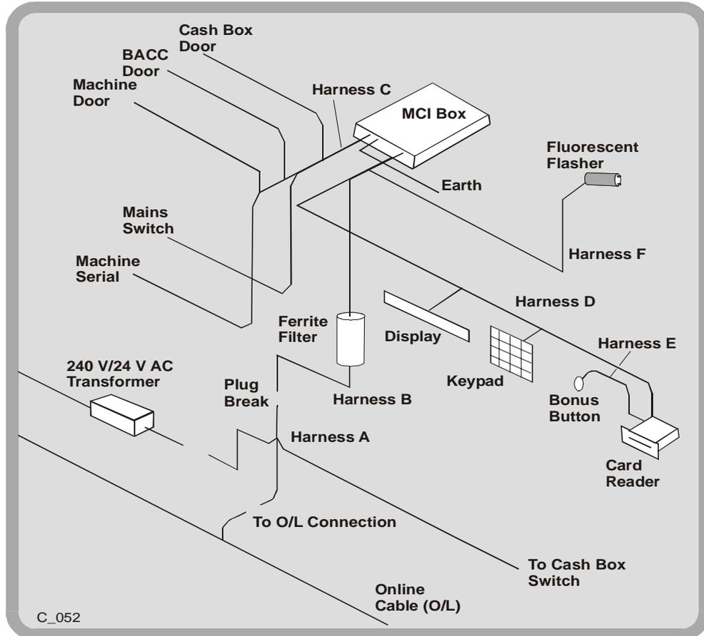
Figure 16-7 MCI - Typical Connections
