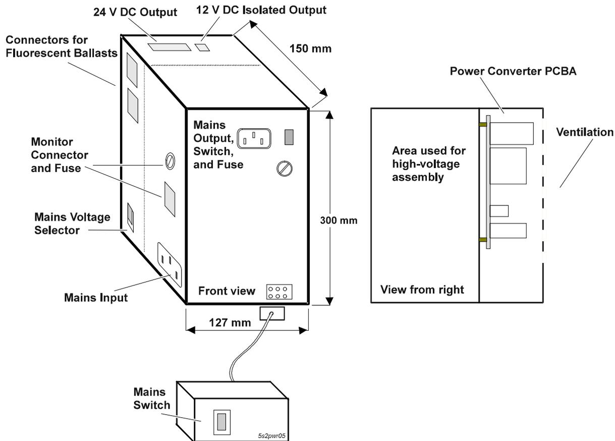
Figure 5-2 Power Supply Assembly
