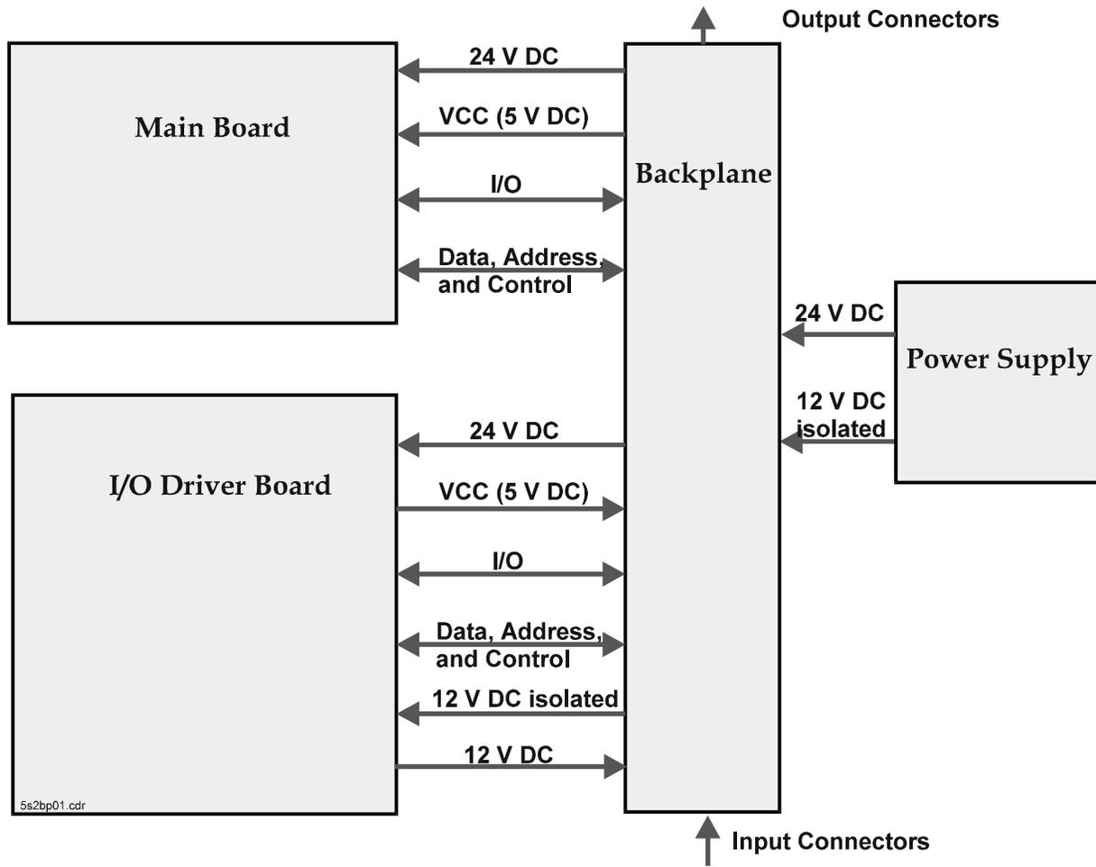
Figure 13-3 System Architecture
