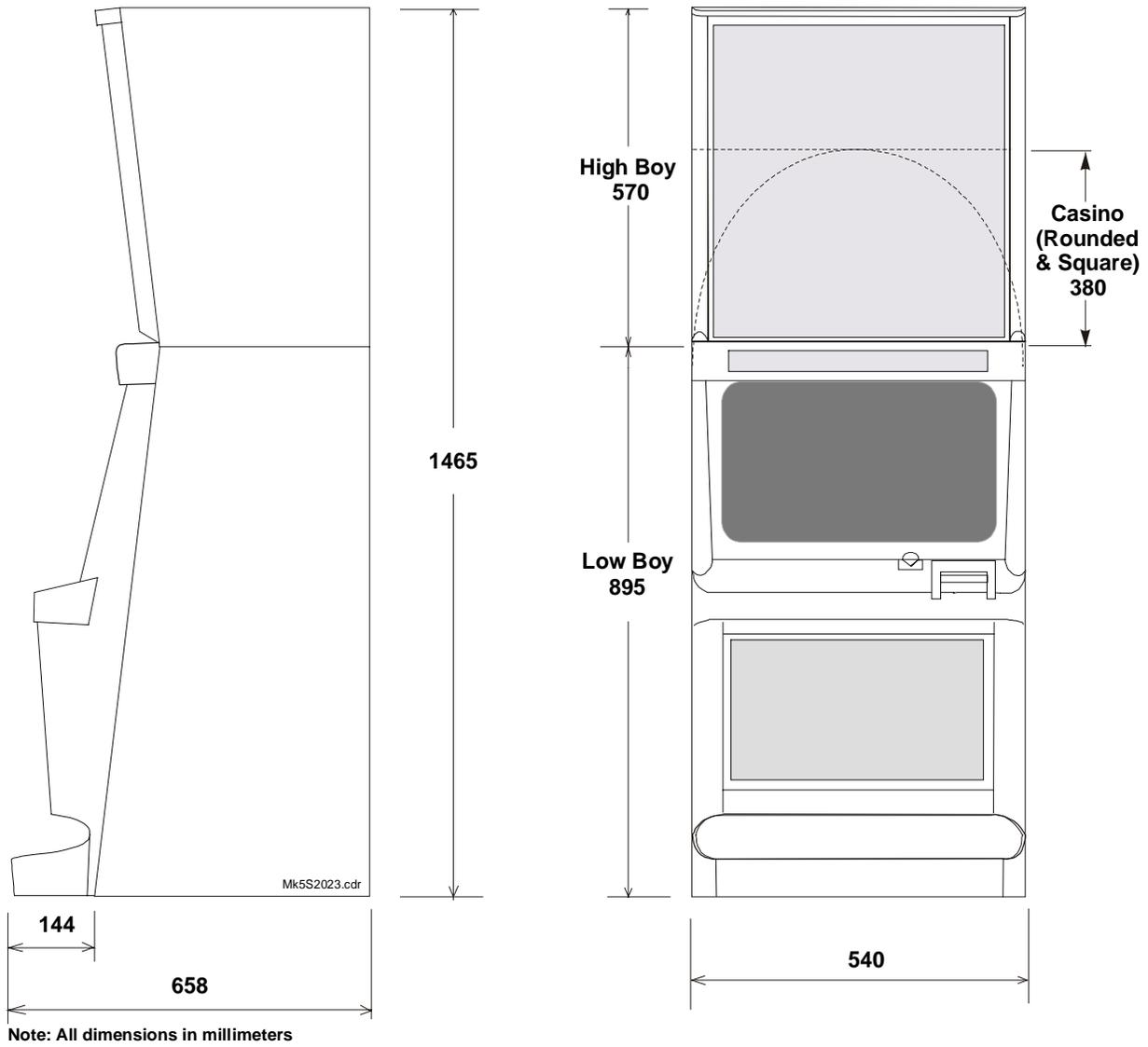
Figure 2-1 Machine Dimensions
