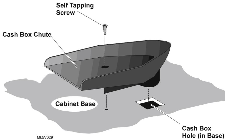
*Figure 4-4 Cash Box Chute: Removal and Replacement*
