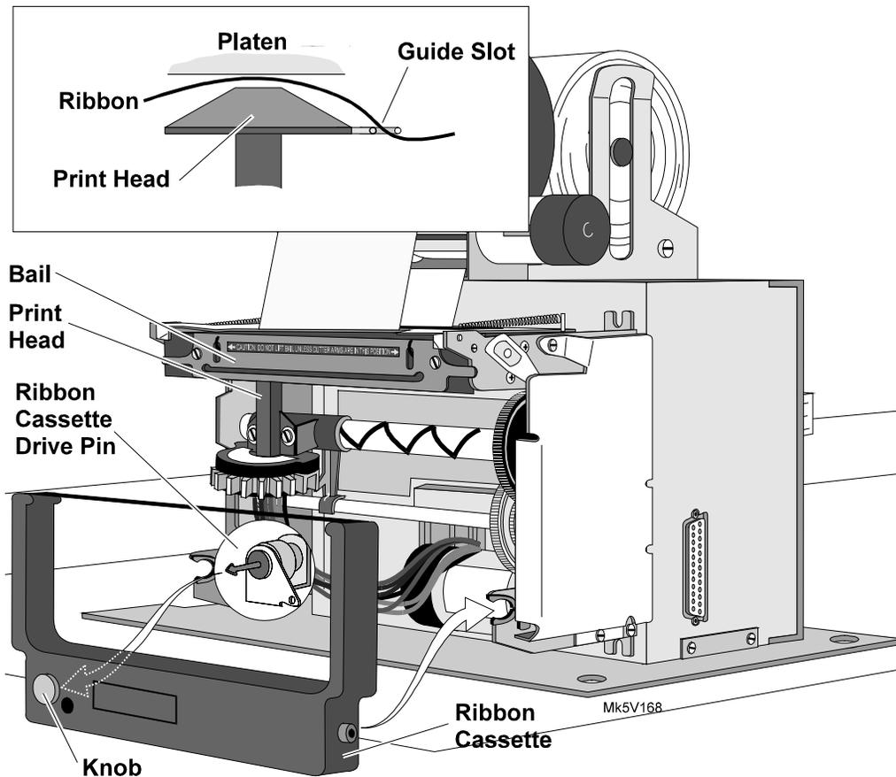
Figure 8-5 Replacing the Ribbon Cassette
