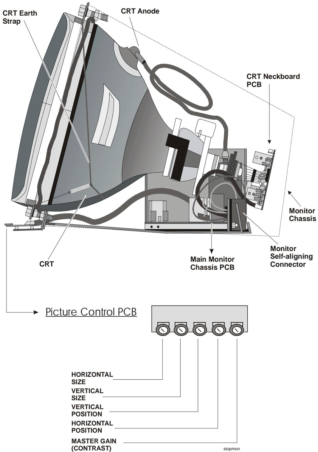
Figure 10-2 Monitor Assembly – Kristel and Ceronix
