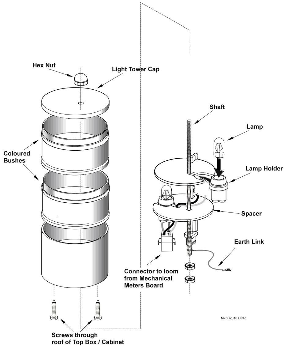
Figure 4-10 Two-tier Light Tower - exploded view.
