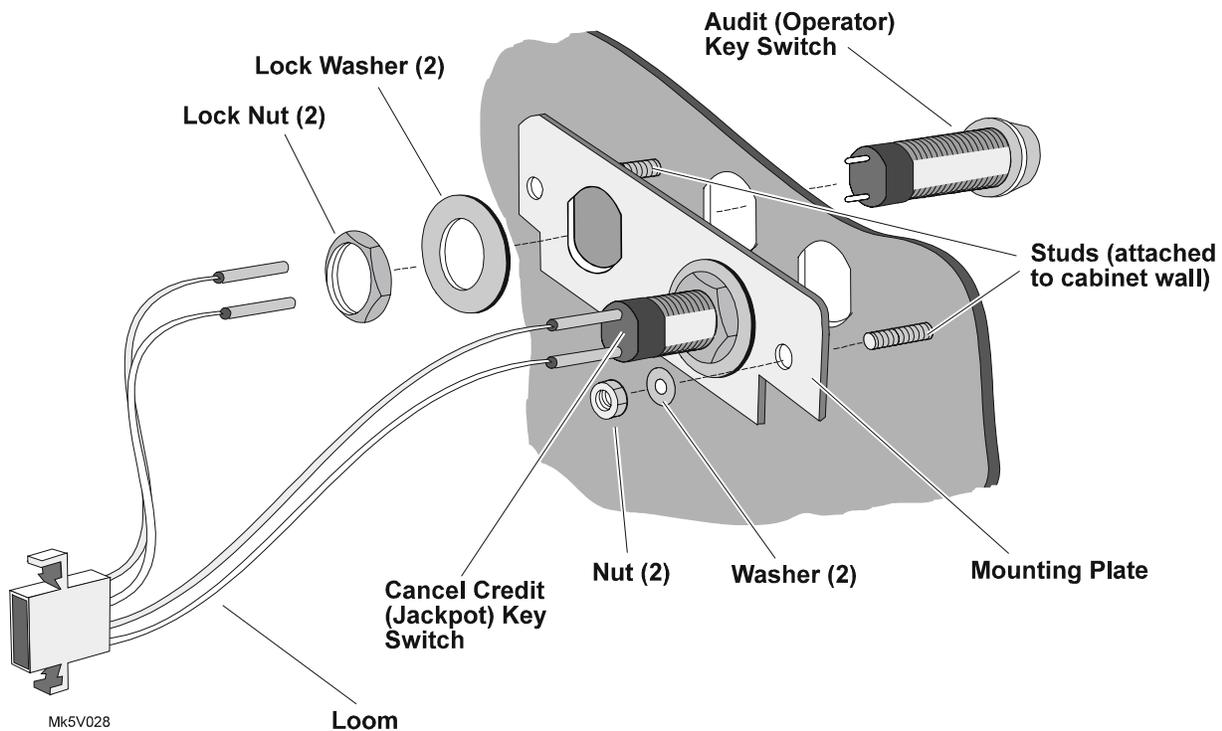
Figure 4-3 Key Switches: Removal and Replacement
