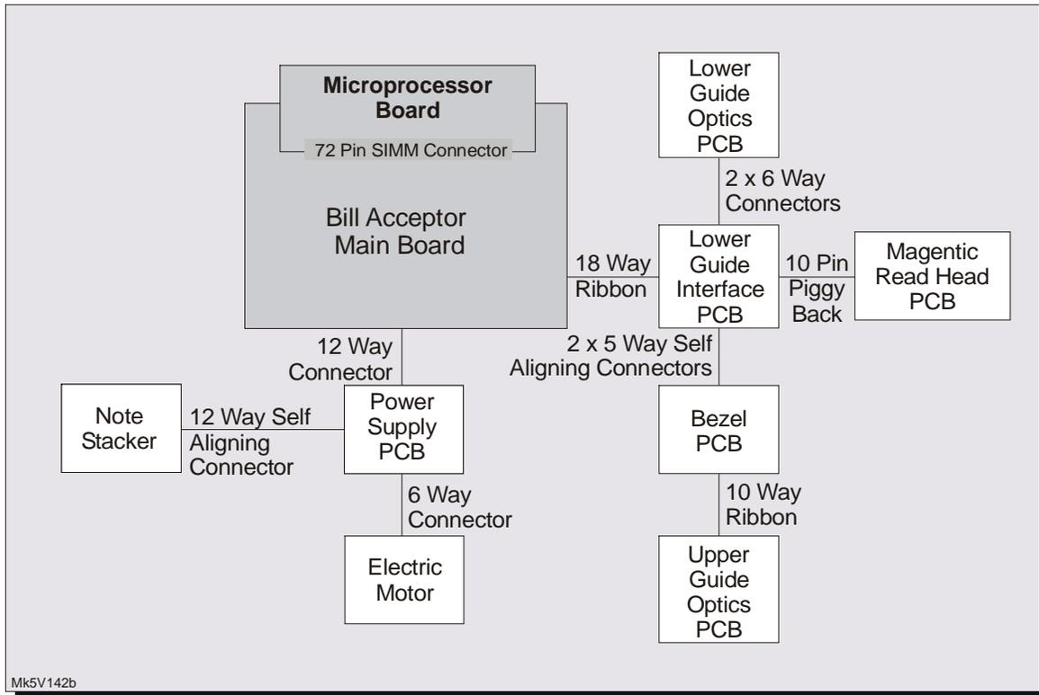
Figure 9-5 Interconnection Diagram
