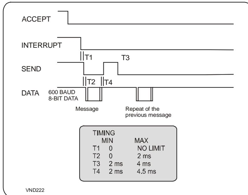
Figure 9-8 GL5 Protocol - Request for Re-transmission Message
