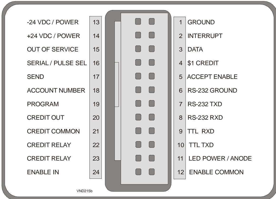
Figure 9-4 Input/Output Connector
