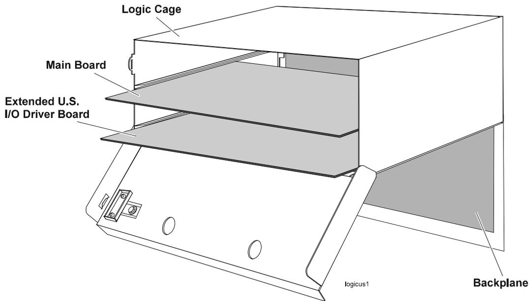
Figure 13-1 I/O Driver Board - Location
