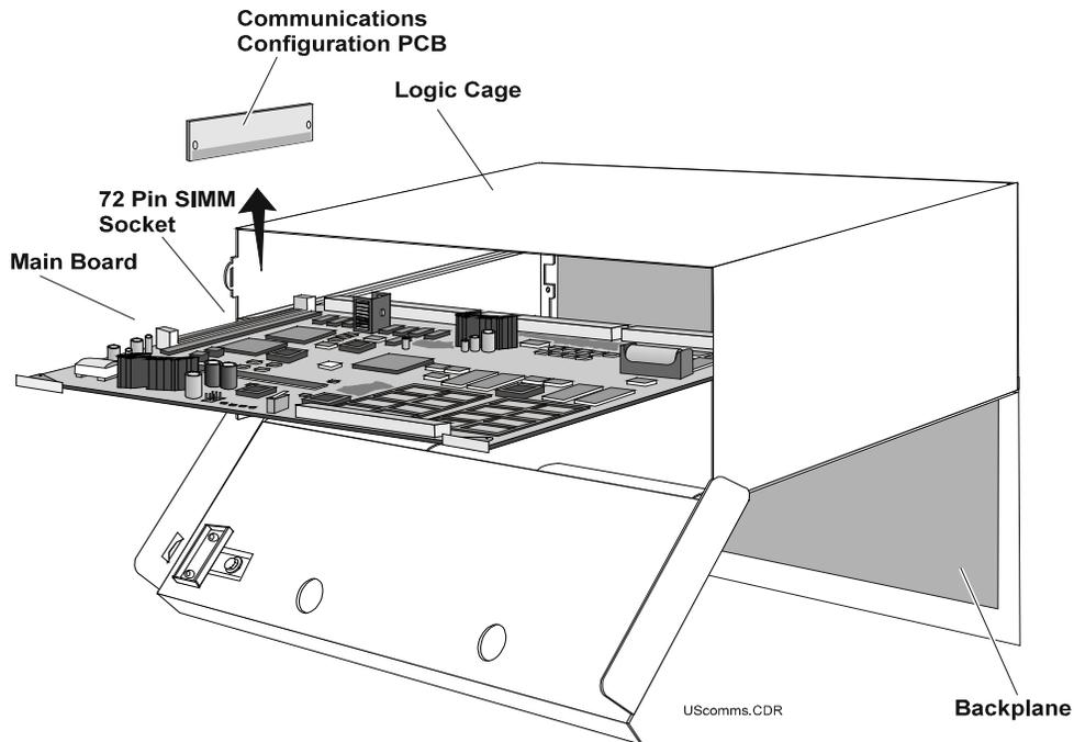
Figure 14-1 Communications Configuration Board - Position in the Logic Cage
