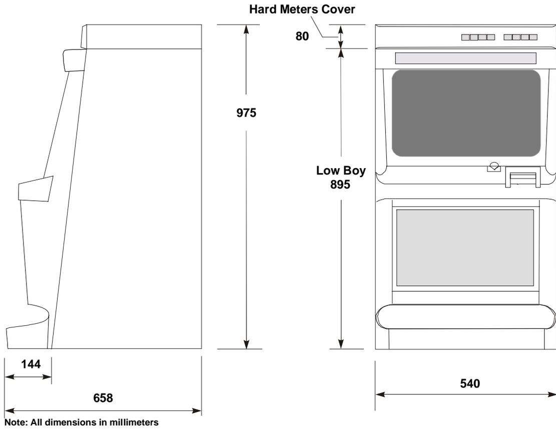
Figure 2-2 Machine Dimensions - Low Boy with Hard Meters
