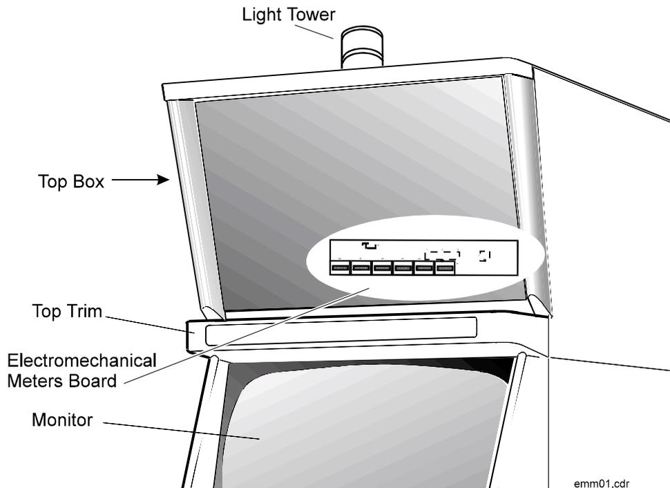
Figure 15-1 Electromechanical Meter Board - Location
