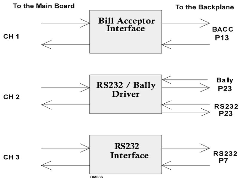
Figure 14-3 Communications Configuration Board - Block Diagram
