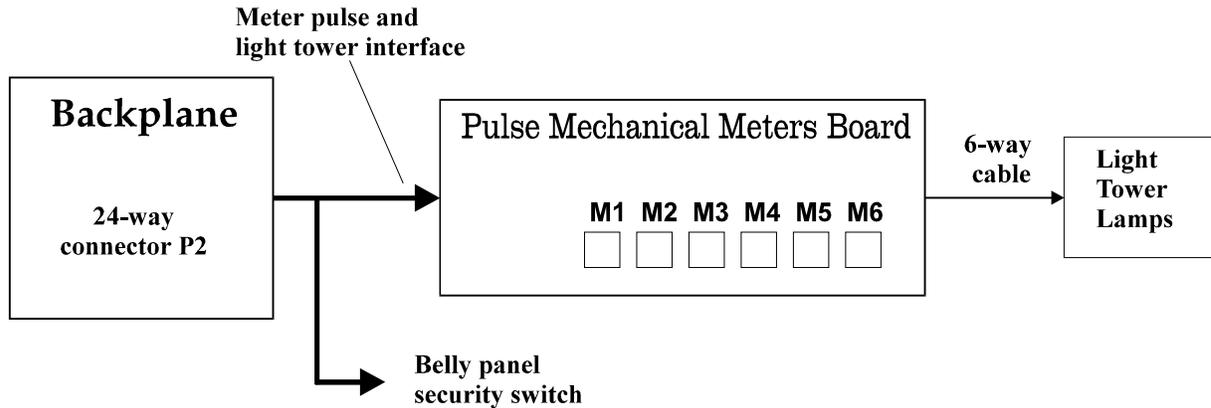
Figure 15-3 Electromechanical Meter Board - Block Diagram
