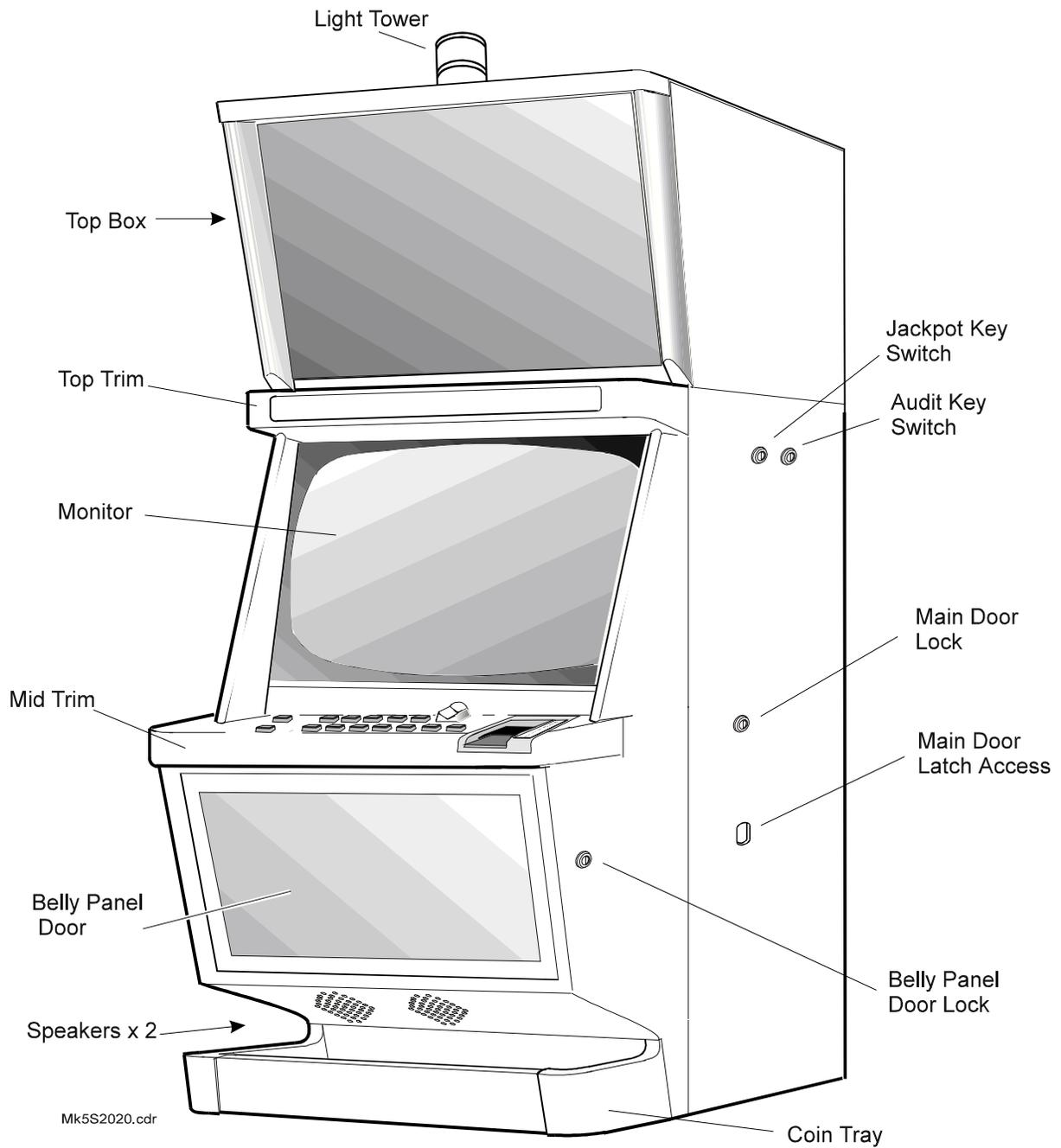
Figure 4-1 MVP Gaming Machine with Highboy Top Box and Bill Acceptor
