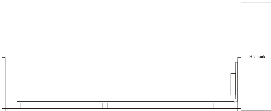
Figure 15-3 Mounting of the PCB and Amplifier Chips to the Chassis
