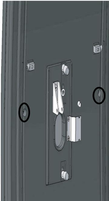
5. Remove the two screws at the bottom of the playfield
