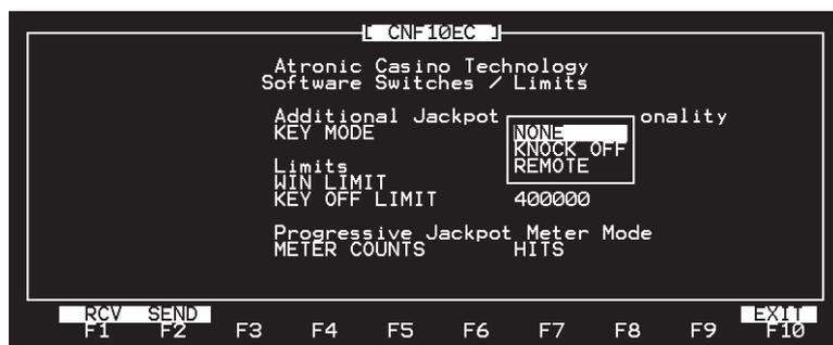
This routine allows the definition of additional functions for the Jackpot Key, to enable or disable the win limit, to set a key off limit and to set the Jackpot Meter mode.
