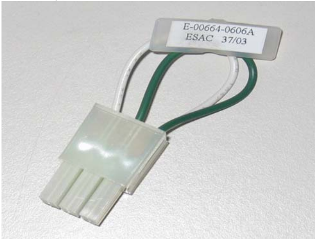
Printer Bypass Jumper, E-00664-0606
