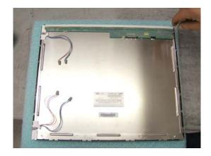
A warning first, the ribbon and PCB board is fragile use <u>caution</u> whenever working around them! Remove the three small Phillips screws securing the PCB and ribbon to the back/plane. To remove the back/plane, unclip the sixteen clips around the outer bezel.
