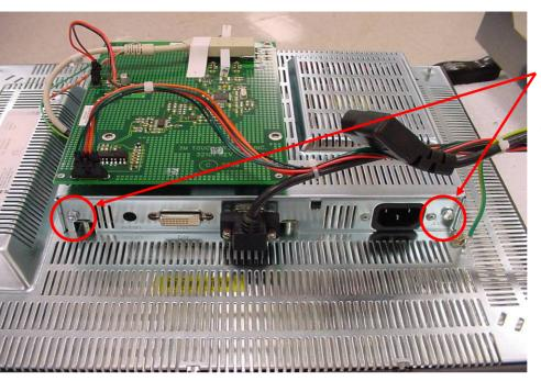
Step 1: Remove the  $2 - \frac{1}{4}$ " drive screws from the back cover. Slide cover back to unlock and remove.
