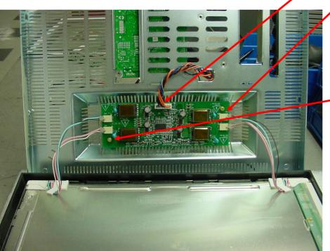
Step 8: remove the 2 phillips screws and install new inverter
