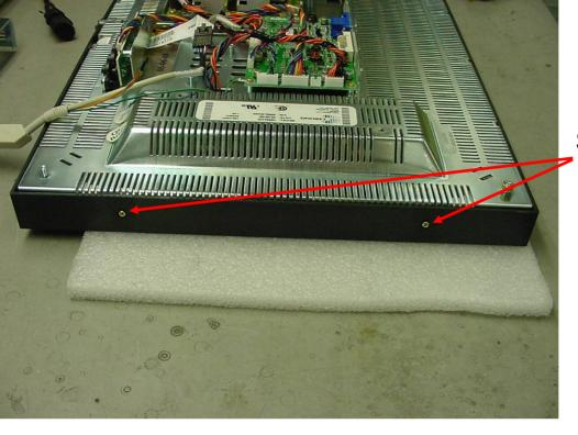
Step 4: Remove the 4 phillips screws from Bezel.
