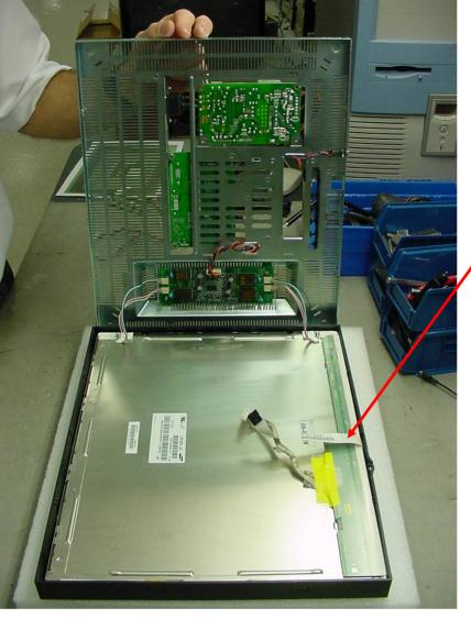
Step 6: separate the LCD from the frame. Use caution not to tear T/S ribbon and inverter lamp wires.
