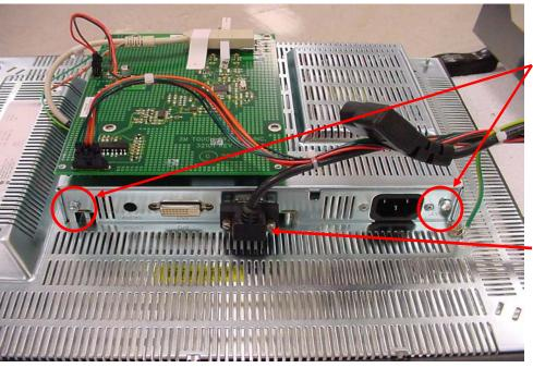
Step 1: Remove the  $2 - \frac{1}{4}$ " drive screws from the back cover. Slide cover back to unlock and remove. Unscrew the 2 nuts Holding the VGA Connector to the A to D board.
