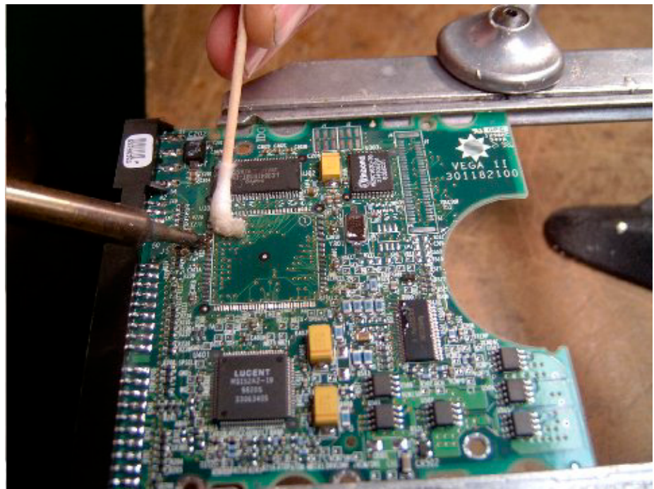
Cleaning of the pads before installing the new chip is important. To clean the pads, use a soldering iron to apply heat while polishing each pad with a swab dipped in flux until thoroughly clean.
