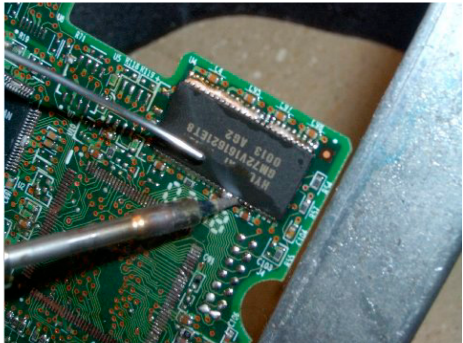
Adding the Chip Quick alloy to the pins of the device to be removed.
