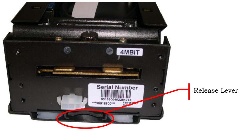
**Figure 3-4** Press the Release Lever
