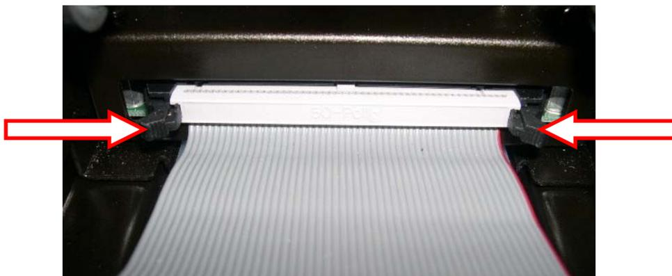
**Figure 3-3 Release the Ribbon Cable**
