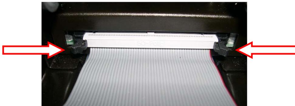
**Figure 3-3 Eject the Ribbon Cable**
