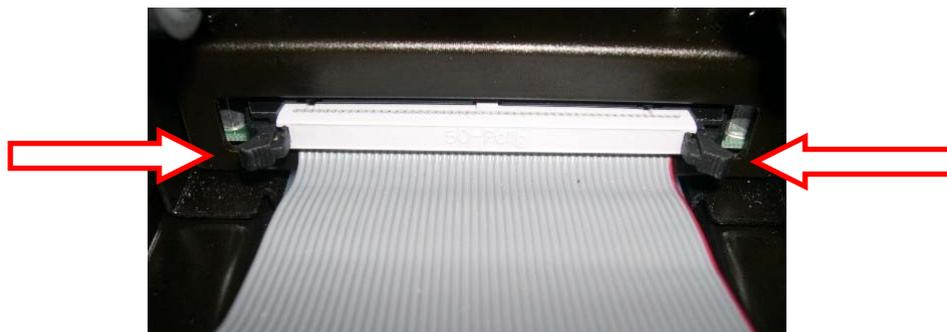
**Figure 2-3** Eject the Ribbon Cable
