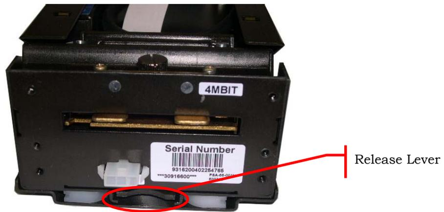
**Figure 3-4** Press the Release Lever
