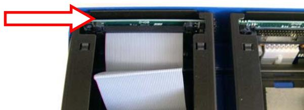
**Figure 3-6** Connect the Ribbon Cable to a Daughter Board
