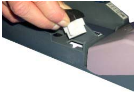
Figure 1-1 Disconnect the Cable
