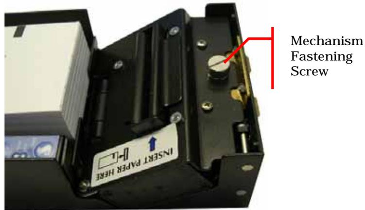
Figure 2-5 Undo the Screw
