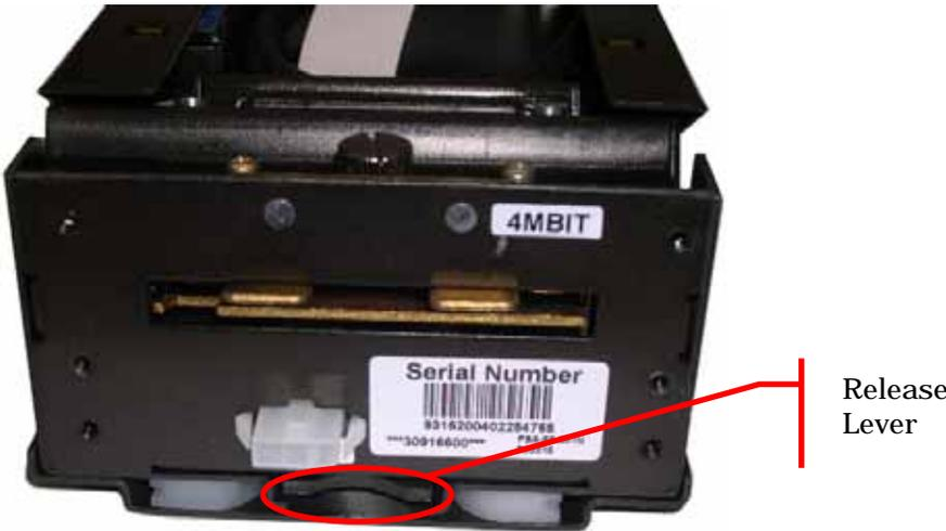
Figure 3-4 Press the Release Lever
