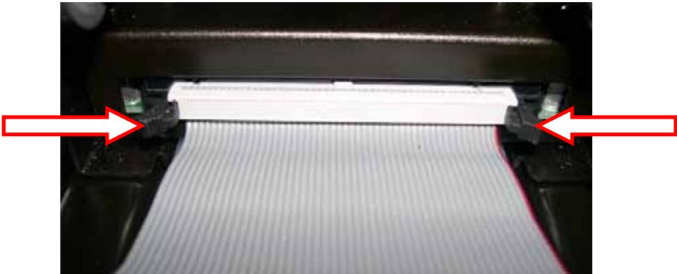
Figure 3-3 Eject the Ribbon Cable
