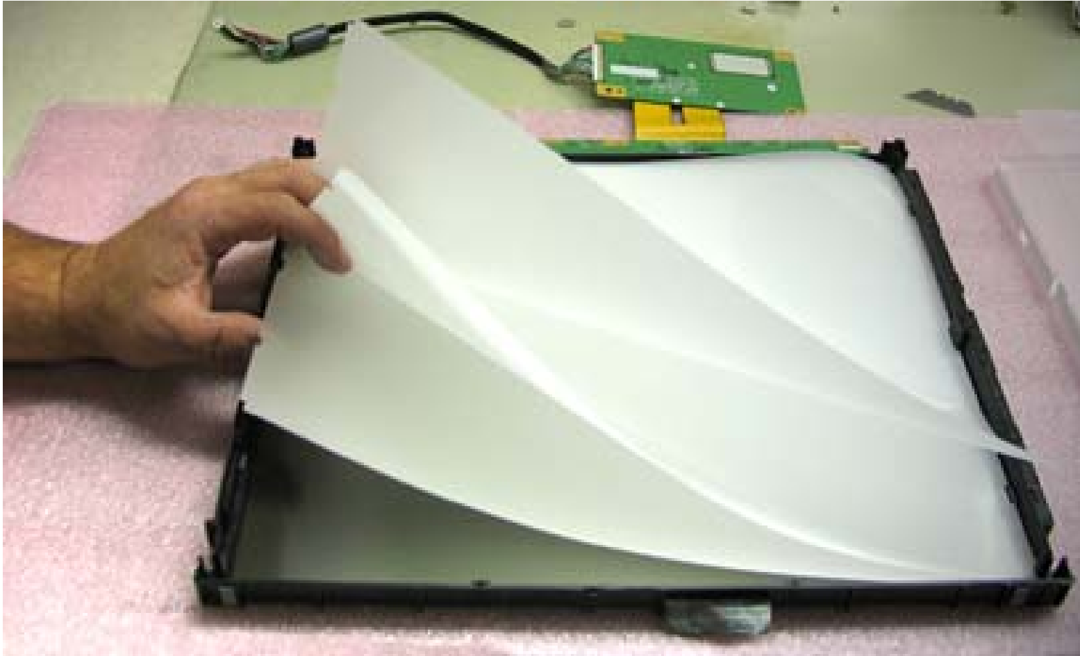
Photo of the Plexiglas plate (right) and film layers in a disassembled LCD panel
