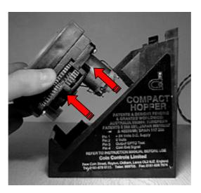
Place the hopper bed assembly face down on a flat, supportive work surface with the disc downwards.
