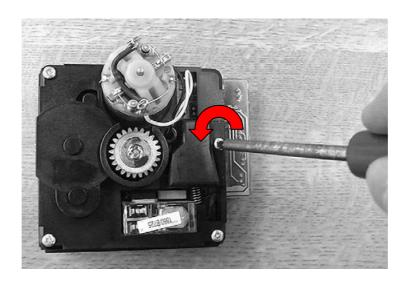
Using a spring hook or similar device, un-hook the ejector spring from the finger by pulling away from the fixed end of the spring and then releasing the tension in the opposite direction.
