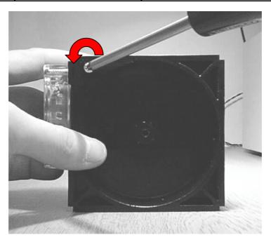
Now fit the new adjuster plate. Most plates (including the Euro) have just one crew hole and so positioning is straight forward. If there are 2 holes in the new adjuster plate, they are referred to as positions 'A' and 'B'. The picture below shows the different locations – use the correct hole for qualified performance. For specific coinage information contact MCL Technical support.
