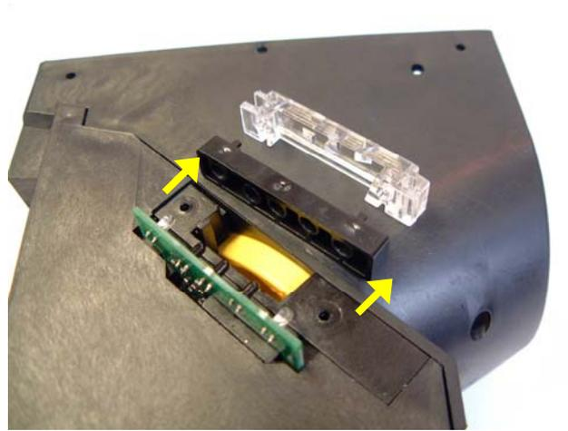
Figure 5: Replace with new light guide Lower section.
