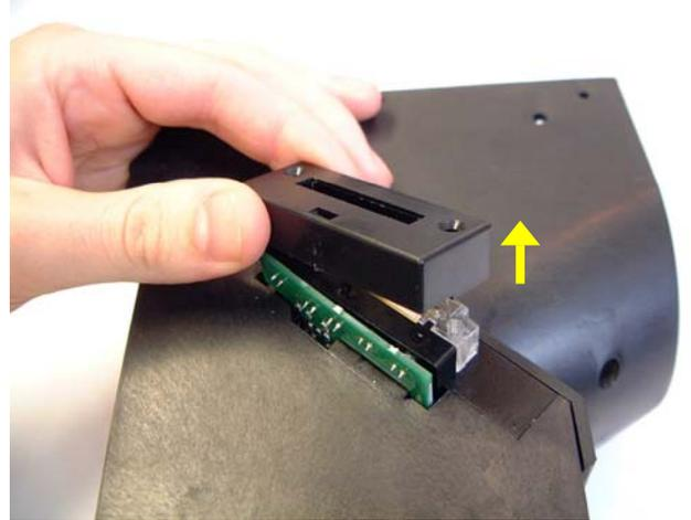
Figure 3: Remove Light guide upper section.
