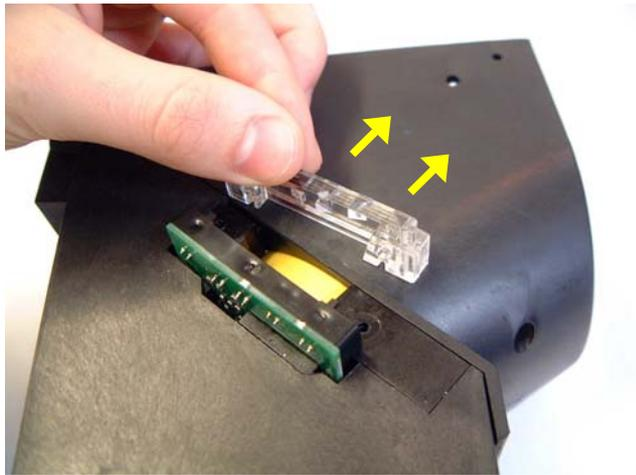
Figure 4: Remove Light guide lower section.
