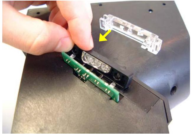
The light guide piece can only be fitted one way, please check the drawing on the right to ensure correct fitting.
