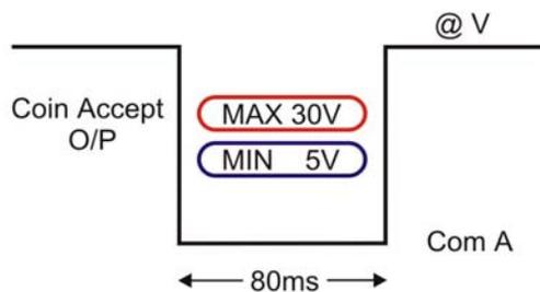
Com A range = -24V to 0V or +5V to +24V
