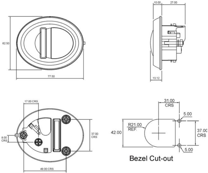
Figure 26: Panel Fixing Dimensions
