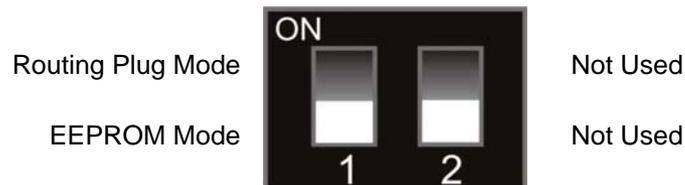
When the desired switch positions are selected press and hold the program button, (situated underneath the rotary switch), the LED will change from Green to Yellow, release the program button; the LED will change back to Green.
