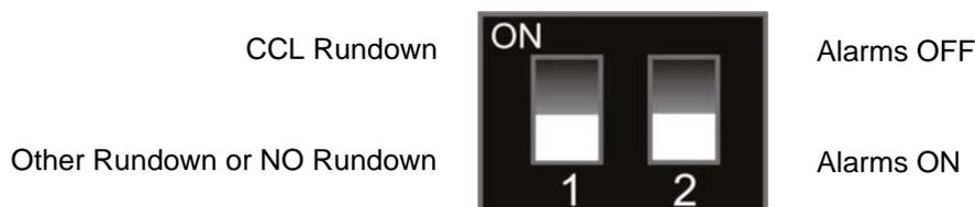
When the desired switch positions are selected press and hold the program button, (situated underneath the rotary switch), the LED will change from Green to Yellow, release the program button; the LED will pulse Red and change back to Green.
