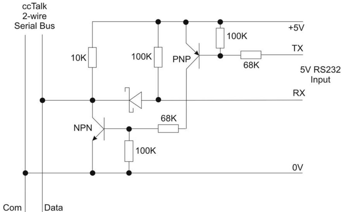
Figure 18: Circuit 1, **ccTalk** Standard Interface
