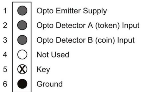
This interface is used with the dual coin rundown. It is used to provide information to the SR5i indicating whether a coin or a token has been entered.
