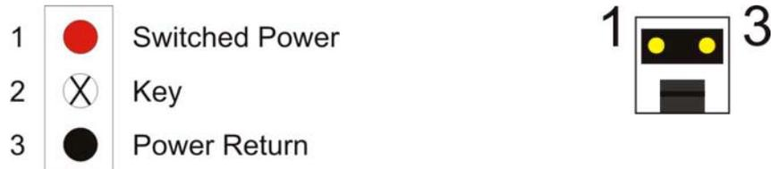
This two pin connector is switched to operate the diverter flap within the active manifold when required as part of 8 way coin sorting.
