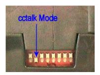
To operate Lumina in cctalk mode, ensure that the device powers up with DIP switch 7 in the ON position. All other switches MUST BE OFF.
