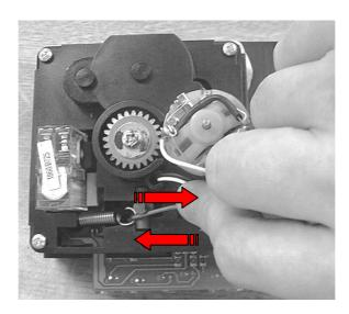
Now pull the spring to one side so that it does not impede the removal of the ejector.
