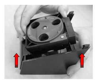
Place the hopper bed assembly face down on a flat, supportive work surface with the disc downwards.
