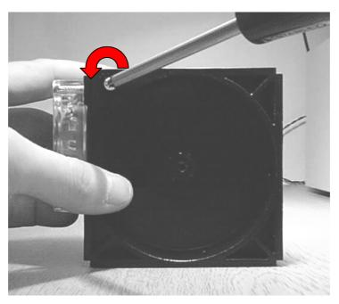
Now fit the new adjuster plate. Most plates (including the Euro) have just one screw hole and so positioning is straight forward. If there are 2 holes in the new adjuster plate, they are referred to as positions 'A' and 'B'. The picture below shows the different locations – use the correct hole for qualified performance. For specific coinage information contact MCL Technical support.
