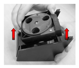
You now have access to the disk. Using a Torx or Pozi-Drive No. 2 screwdriver, turn the central screw anti-clockwise to loosen and remove the screw.
