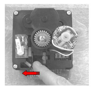
Undo the screw completely as shown below.
