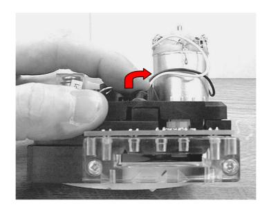
Then, whilst gripping the tip of the ejector finger (shown above) turn the hopper over and push out the fingers from its locating holes until they are moving freely.
