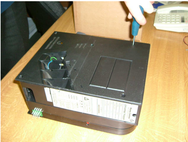
Figure 3: Remove coin box screws (5 off).
