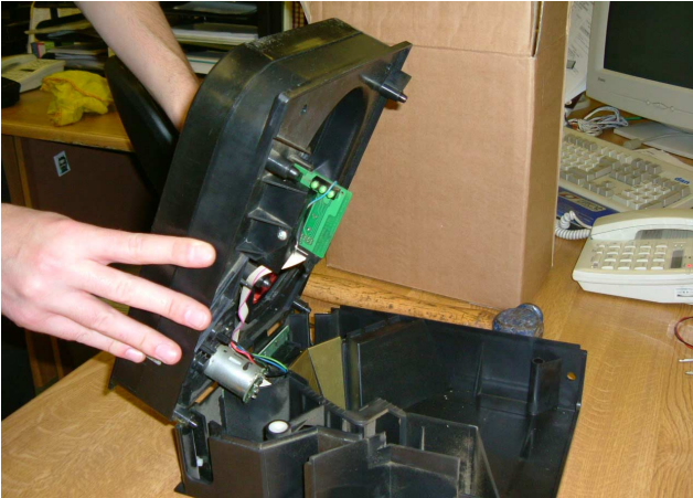
Figure 13: Close Hopper, ensuring cables are free.
