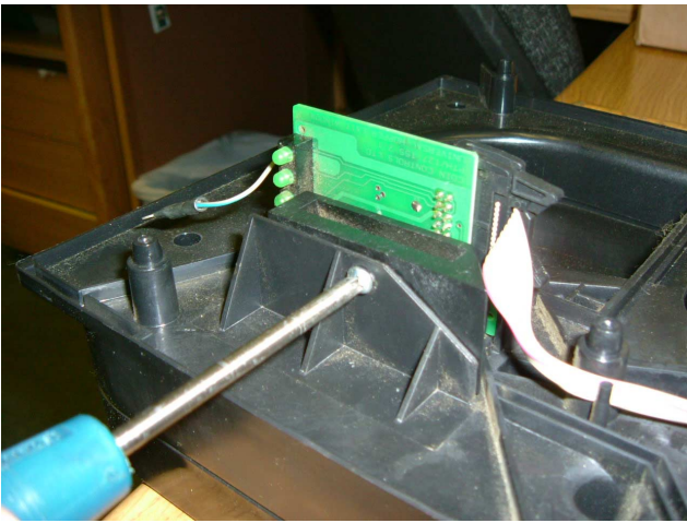
Figure 11: Replace spacer screw.
