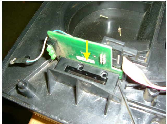
Figure 8: Slot back into centre plate.
