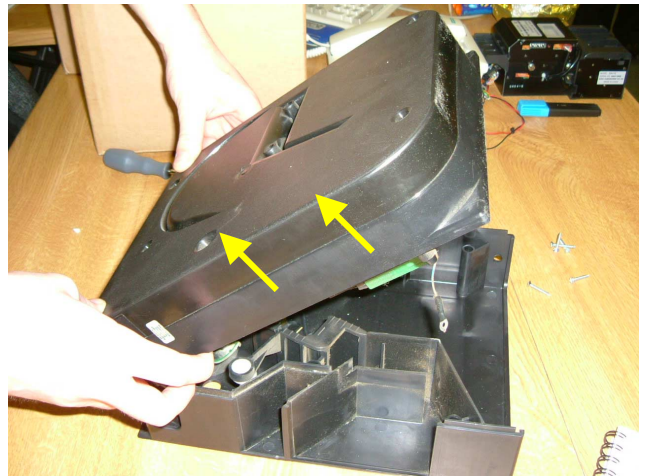
Figure 4: Turn hopper over and open.
