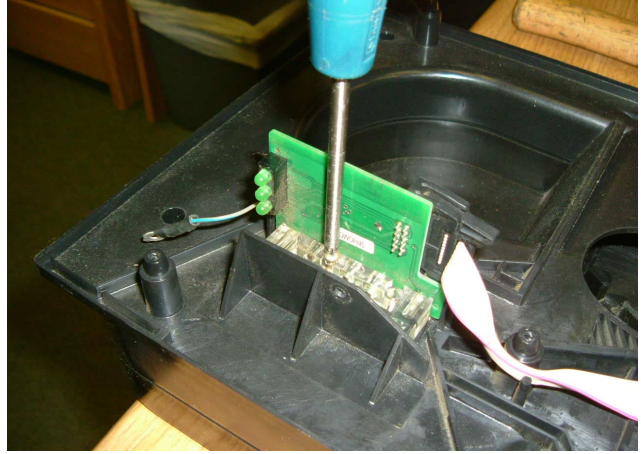
Figure 6: Remove light guide screws (2 off) and slide out light guide.
