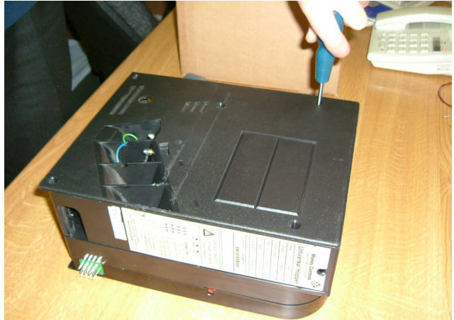
Figure 14: Turn hopper over and replace coins box screws.
