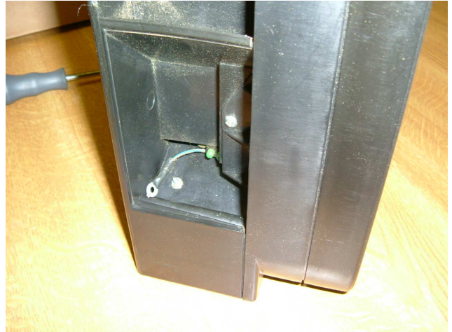
Figure 2: Remove level sense wire.
