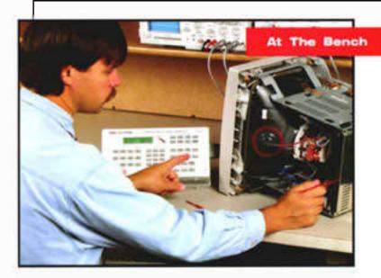
The CM125 "Pix Pak" Computer Signal Monitor Generator is the perfect instrument for bench troubleshooting. It packs a powerful pixel punch with 125 MHz video bandwidth and 2048 X 2048 resolution. Complete parameter programmability and video patterns help you effectively test the high resolution monitors that come across your bench.
