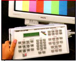
Portable computer monitor signal generator for monitor testing at the bench, the burnin rack, or in the field.
