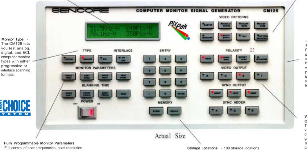
(up to 2048 x 2048) and blanking time parameters let you setup the output of the CM125 to match the input requirements of your monitor under test. **Storage Locations** - 100 storage locations (43 preprogrammed) let you quickly store and recall the most common monitor formats you test.
