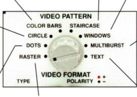
Multiburst: This pattern tests monitor resolution and bandwidth. The vertical lines test the horizontal pixel resolution and the horizontal lines test the vertical resolution. The one pixel wide line should be discernible on a property operating monitor.
