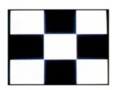
Windows: Use this pattern to test the monitor's power supply regulation. Check for a clear, distinct transition between the black and white portions. All the white boxes should be the same brightness level and the entire screen should be free of any ripple.
