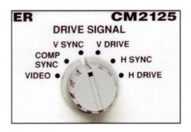
The CM2125 uses the signal substitution troubleshooting technique to isolate problems in less than half the time you now take. Signal substitution helps you narrow the problem down to a single stage by injecting a known good signal into the input of a functional block (seen below) and monitoring the output or the CRT. If the output is OK (a clear, locked-in picture on the dis-
