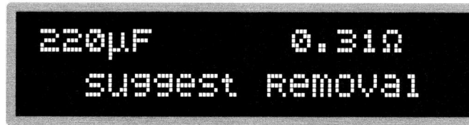
Fig. 5: The "SUGGEST REMOVAL" readout indicates there are components in parallel with the capacitor being measured that will influence the test results.
